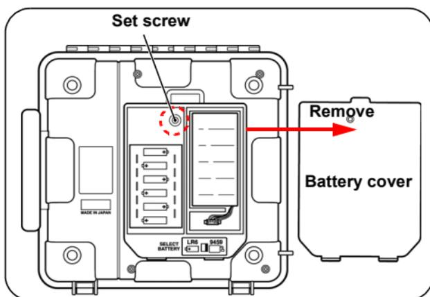
3. Disconnect the plug of the battery pack from the connector of the instrument.
