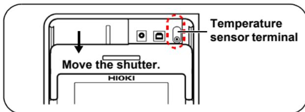
2. Connect the temperature sensor to the temperature sensor terminal.
