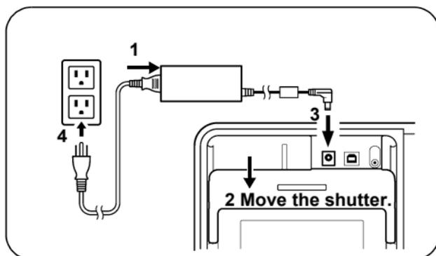
1. Insert the power cord into the AC adapter.
