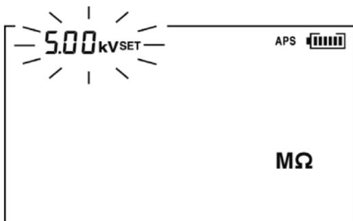
6. The test voltage is chosen from 250 V, 500 V, 1.00 kV, 2.50 kV, and 5.00 kV using the
