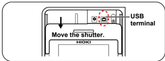
2. Connect the USB Cable to the USB terminal.
