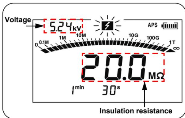
8. Stop insulation resistance measurement.
