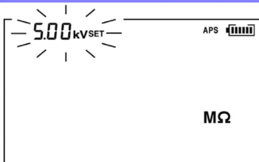
5. Press the
