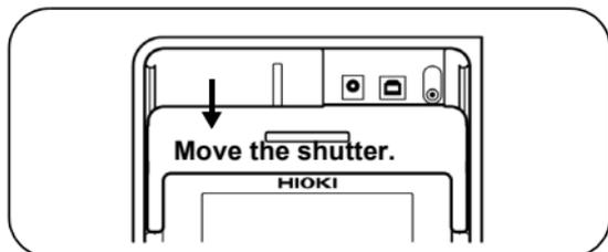
3. Connect the AC adapter to the AC adapter terminal.
