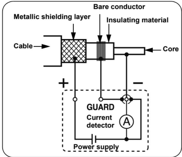
When testing the insulation of a cable, as shown in the diagram above, wind a bare conductor around the surface of the insulating material and connect the conductor to the GUARD terminal. This prevents the leakage current on the surface of the insulating material flowing into the current detector, which enables the actual resistance of the entire volume of the insulating material to be measured.
