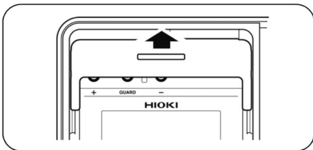
3. Connect the red test lead to the + terminal and the black test lead to the - terminal. Connect the blue test lead to the GUARD terminal if necessary. Fully insert the test leads.
