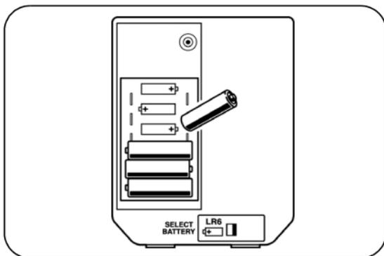
4. Turn the battery selector switch to LR6. When the power is turned on, “LR6” appears on the top left of the screen.
