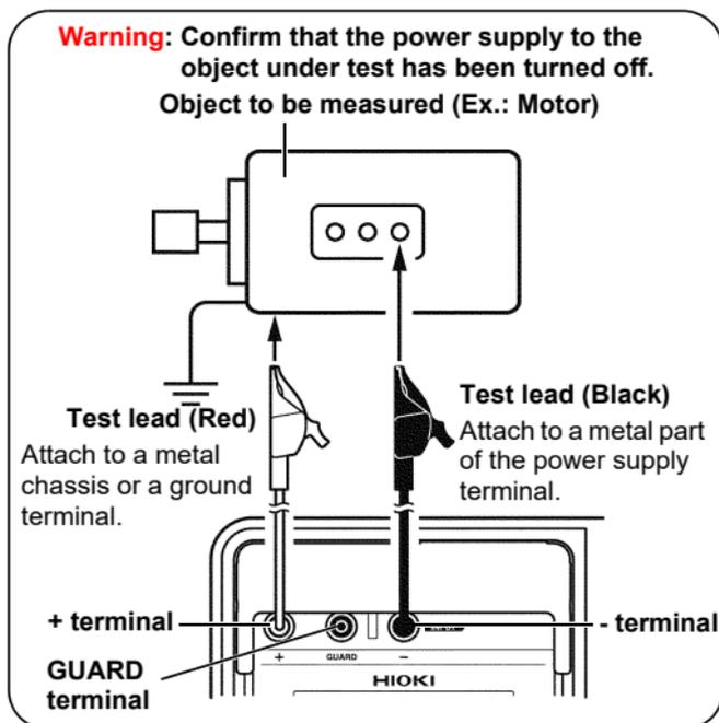
4. Clip the alligator clip at the end of each test lead to the object under test.
