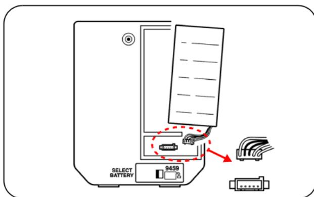
4. Connect the new battery pack to the instrument. (Align the protrusions.)
