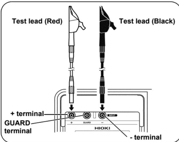
4. Clip the ends of the test leads to the circuit to be tested. When the voltage exceeds 50 V, the
