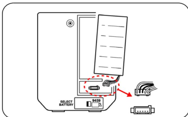
4. Place the battery pack in the battery pack compartment.
