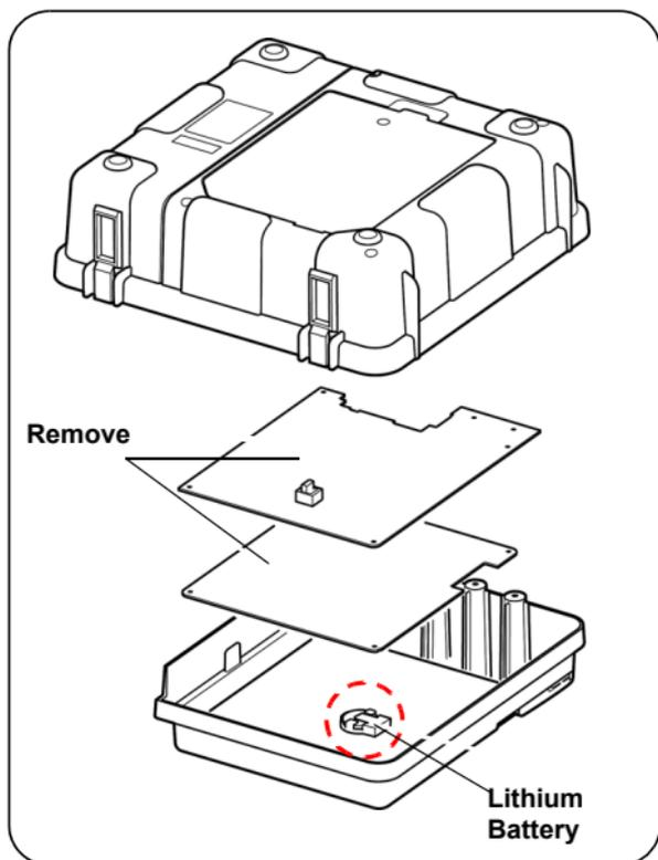
4. The battery is located on the remaining PCB as shown in the illustration on the previous page.
