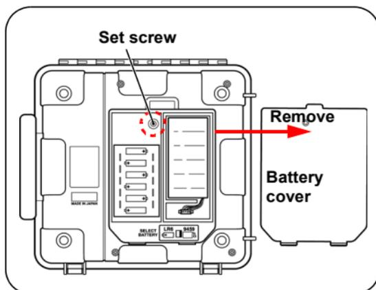
3. Place six LR6 Alkaline batteries or six HR6 Nickel-metal hydride batteries into the battery compartment. (Replace all six at the same time)
