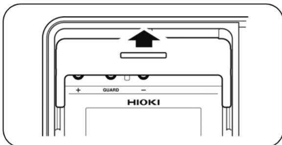
3. Connect the red test lead to the + terminal and the black test lead to the - terminal. For insulation resistance measurement, connect the blue test lead to the GUARD terminal if necessary. Check that the test leads are fully inserted.
