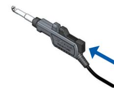
2. Clamp the hook around the cable whose signals you wish to detect and release the open/close lever.
