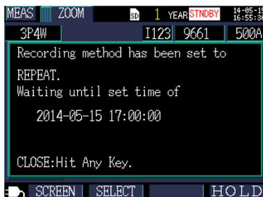
Recording will be started at the start time on the set start date. (The recording LED will light up.)
