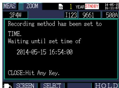
When the set start time is reached, recording will start (and the recording LED will light up).
