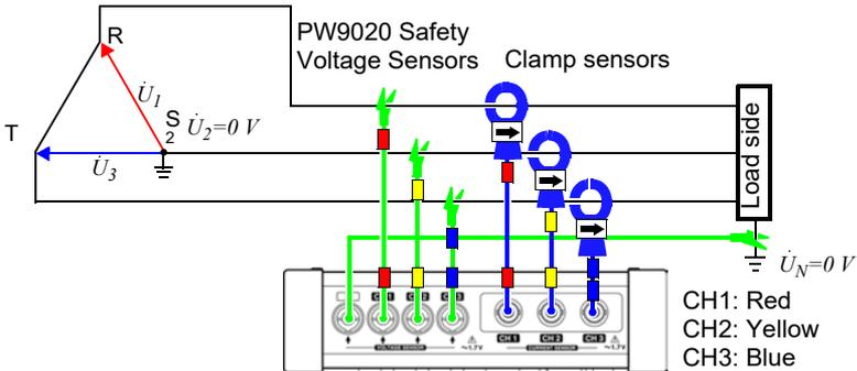
U2 will become 0 V, causing a voltage input fail. (Depending on the installation environment, it may not become 0 V.)
