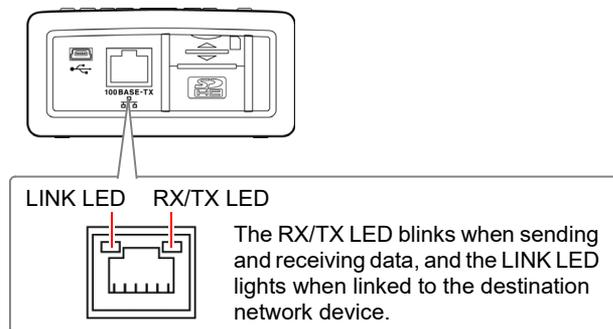
**When connecting the instrument to an existing network
