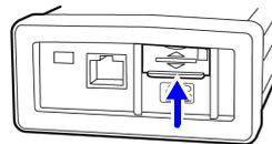
To remove the card, open the cover and push in the SD memory card.
