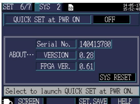
**Start Quick Set at power-on [QUICK SET at PWR ON]**
