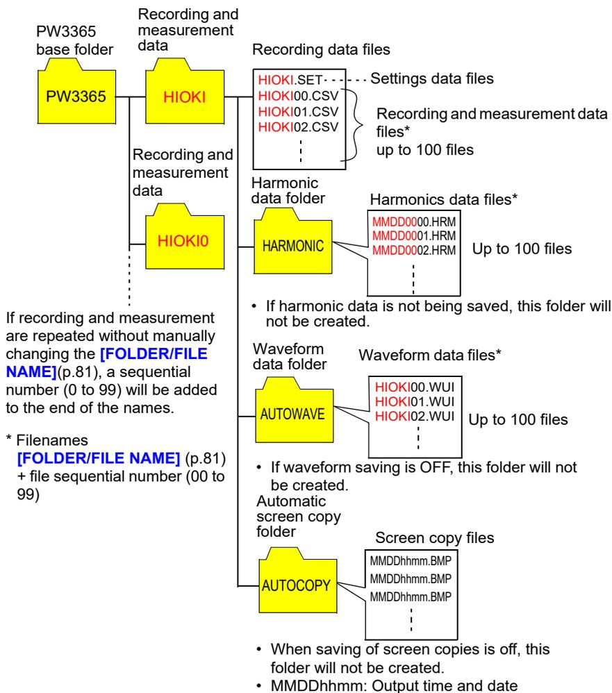
**Reference** When one of the recording and measurement data file, harmonic data file, or waveform data file exceeds 200 MB, all the files will be segmented and new files added.
