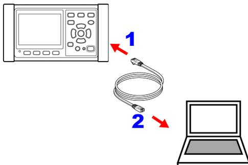
**Reference** Since the instrument provides functionality for automatically detecting whether a straight or cross cable is being used, a straight cable may also be used. If you are unable to establish communications with the computer, try a cross conversion cable (Model 9642 accessory).
