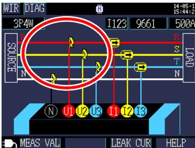
Connect the voltage sensor to the measurement target while checking the wiring target on the [\[WIR, DIAG\]](#) screen.
