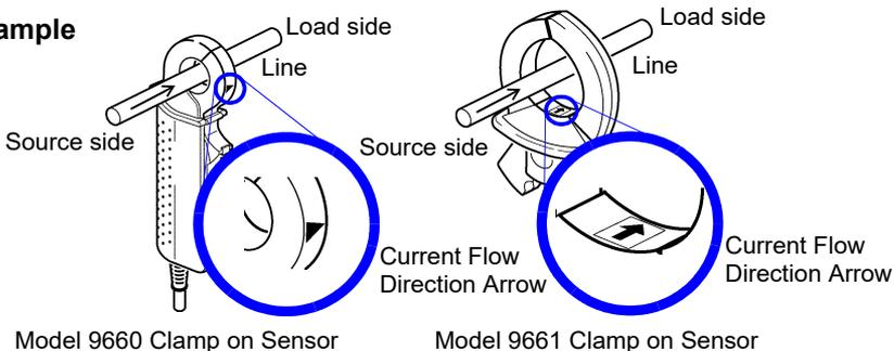
Attach the clamp around only one conductor. Single-phase (2-wire) or three-phase (3-wire) cables clamped together will not produce any reading.
