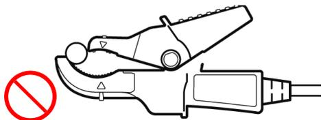
Clamped with the measurement target at an angle
