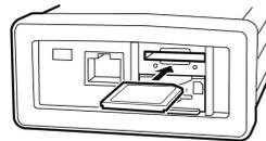
Keep the card level as you insert it. Inserting it at an angle may cause the write-protect lock to engage, preventing data from being written to the card.
