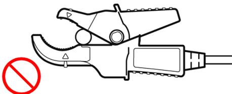
Clamping targets with different voltages at the same time
