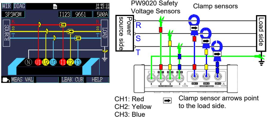
Three-wattmeter measurement with the PW3365
