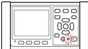
Flashing recording LED
