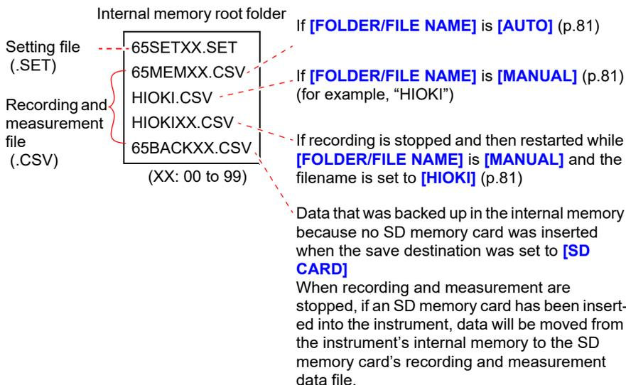
**Reference** The maximum number of files that can be created in the instrument's internal memory is 100. Attempting to create more than 100 files will result in an error.
