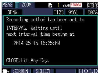
Recording will start automatically when a good time division is reached based on the save interval time. (and the recording LED will light up).
