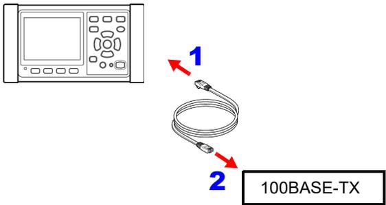
**When connecting the instrument directly to a computer
