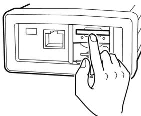
**3** Insert the SD memory card into the SD memory card slot on the computer.
