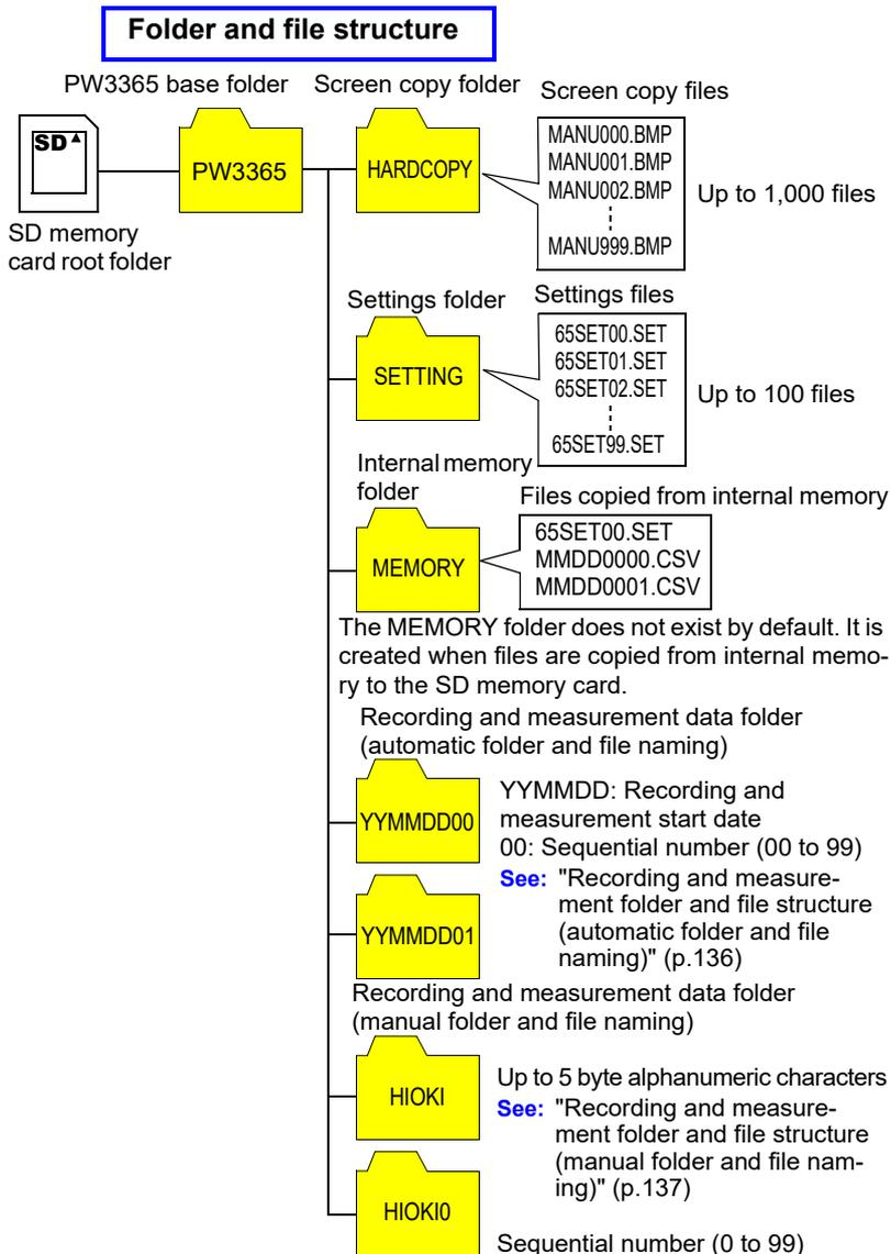
**Reference** • Recording and measurement data files, harmonic data files, and waveform data files are stored in the recording and measurement data folder. When one of the size of them exceeds 200 MB, all the files will be segmented and new files added.
