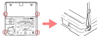
Pass the ring on both ends of the supplied strap through each of the four holes in the instrument.
