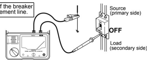
\*When measuring an insulation resistance that contains a capacitance element, a charge proportional to the measurement voltage accumulates, and if undischarged could lead to an electric shock accident.
