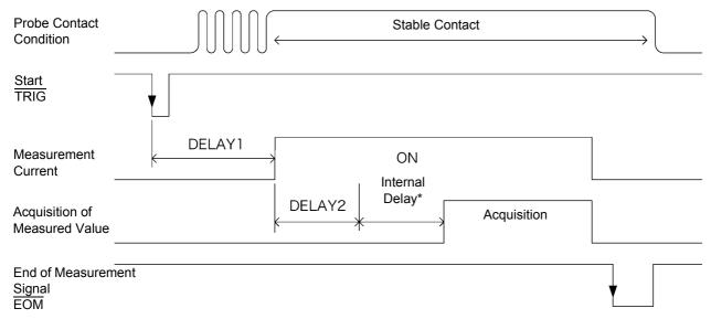
\* Internal delay is provided to suit purely resistive (non-reactive) DUTs, and is different for each measurement range.
