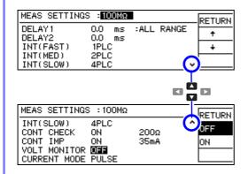
Shows detailed settings for measurements. Adjust the measurement speed, stability and measurement fault detection functions.
