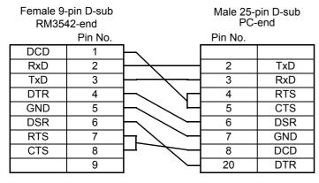
Note that the combination of a dual male 25-pin D-sub cable and a 9- to 25-pin adapter cannot be used.
