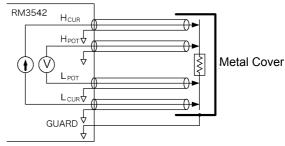
Figure 2. For High-Resistance Measurements
