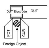
When a probe short-circuit is detected, an error message appears on the measurement screen, and the  $\overline{PRB\_SHORT}$  and  $\overline{ERR}$  signals are output. (ERR:021 Probe short error)
