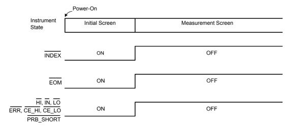
Operation is shown when the trigger source is set to external triggering (EXT).
