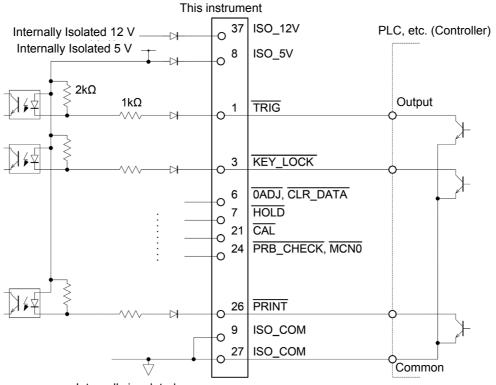
Internally insulated common (Isolated from the protective ground of this instrument.)
