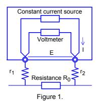
Measurement current I flows through test object resistance  $R_0$  as well as lead resistances  $r_1$  and  $r_2$ .
