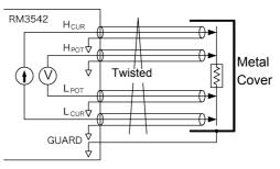
Figure 9. Wiring to Minimize Noise Ingress
