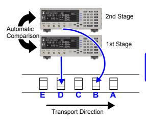
Connect the two instruments' SET MONITOR connectors together using a Hioki 9637 RS-232C cable.
