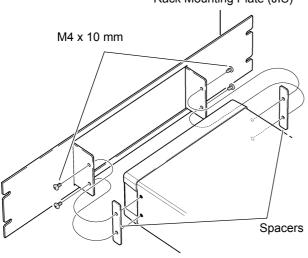
When installing into the rack, reinforce the installation with a commercially available support stand.
