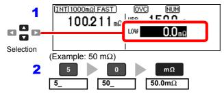
Press the units key to accept the setting and move the cursor to the upper threshold.
