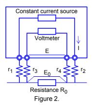
Current I flows from  $r_2$  through DUT resistance  $R_0$  and through  $r_1$ . The high input impedance of the voltmeter allows only negligible current flow through  $r_3$  and  $r_4$ .
