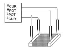
Figure. 11 Four-Terminal Measurement
