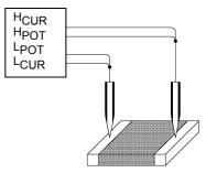
Figure. 10 Two-Terminal Measurement
