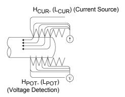
Figure 5. Measurement with Model 9140 4-Terminal Probe
