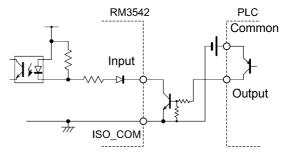
PLC Output (Source Output) Connections
