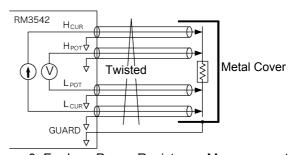
Figure 3. For Low-Power Resistance Measurements
