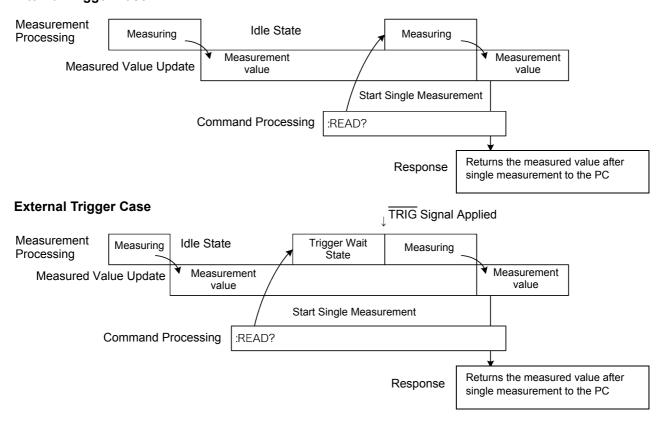
Use this method to measure (and export) synchronously with the PC or external trigger signal. Measurement time can be minimized.
