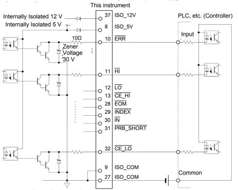
Internally insulated common (Isolated from the protective ground of this instrument.)
