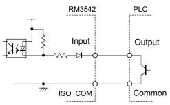
PLC Output (Sink Output) Connections
