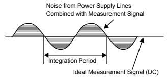
Figure 1. Effect of Noise from Power Supply Lines
