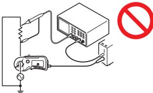
Never connect the device as shown in the illustration.
