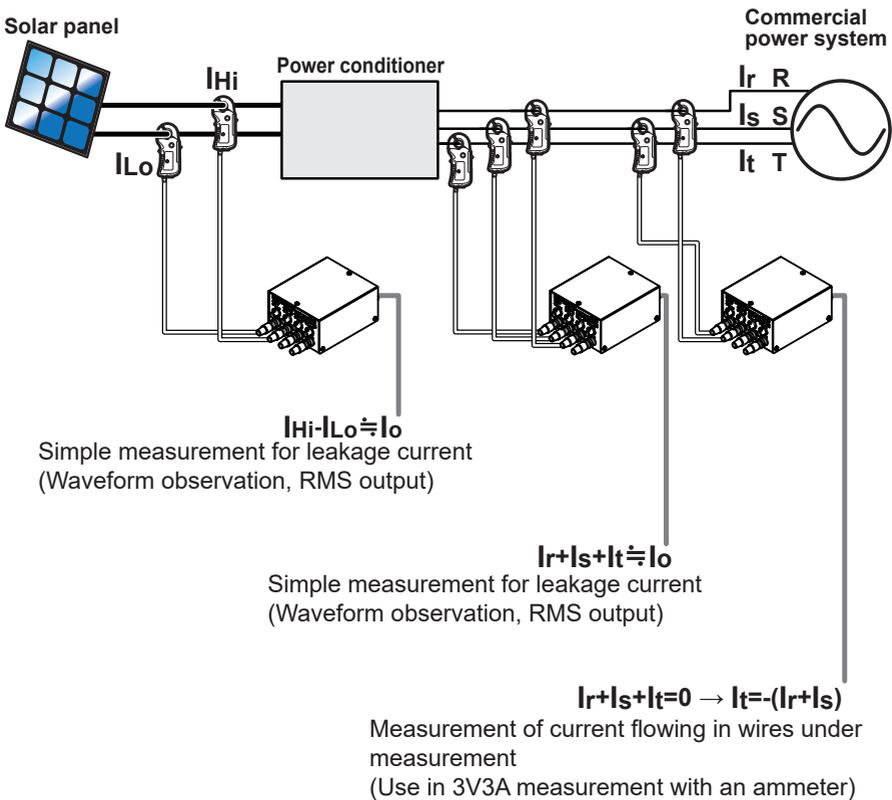
The measurement is affected by errors in each current sensor when measuring the leakage current.
