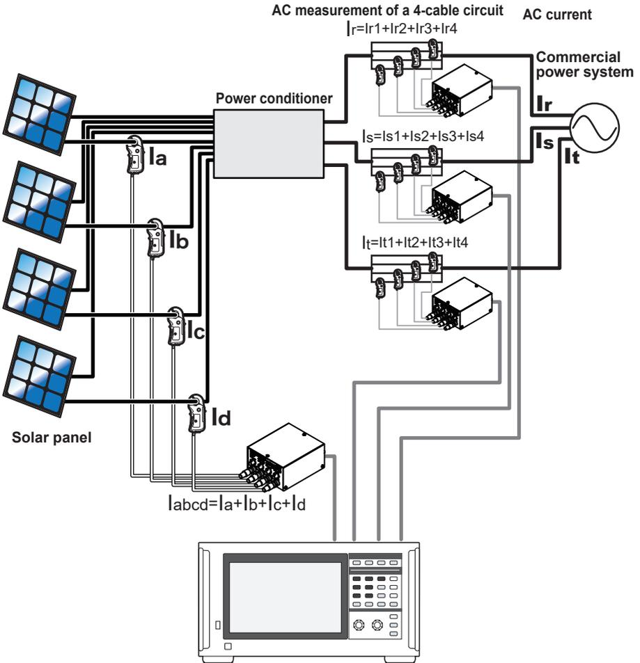
When measuring multiple lines with a total current that exceeds the rated value of the current sensor used, ensure that the conductors adjacent to the current sensor are as far away as possible from the sensor because the current sensor may be affected by the adjacent conductors.
