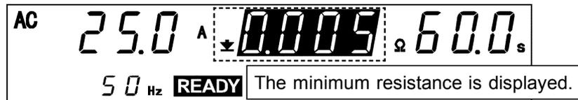
To set a minimum test value, do the same as when setting a maximum test value. The minimum test value must be smaller than the maximum test value. Otherwise, a test will not start when the **START** key is pressed.
