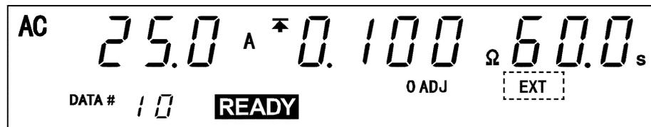
When  $\overline{\text{EXT-E}}$  of the external I/O terminal is at LO, the **EXT** lamp lights to indicate that the external I/O is active.
