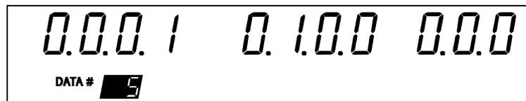
Use the  $\uparrow/\downarrow$  keys to change the maximum value for the number of test data. In this example, press the  $\uparrow$  key four times.
