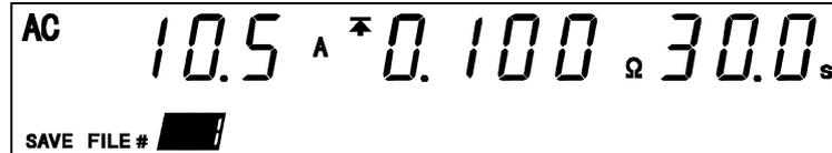
In this status, the preset minimum test valve can be checked by using the **◀** or **▶** key.
