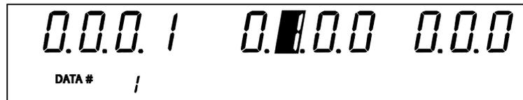
When "Test data count" is activated, the screen shifts to allow you to set a maximum value for the number of test data. In this example, the current maximum number is "1."
