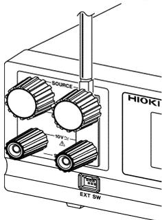
In a test using two terminals, be sure to use the current output terminal.
