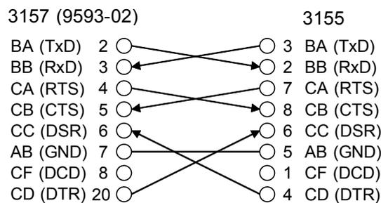
Specification: D-subminiature 25-pin male to D-subminiature 9-pin female connectors, with "crossed" data connections
