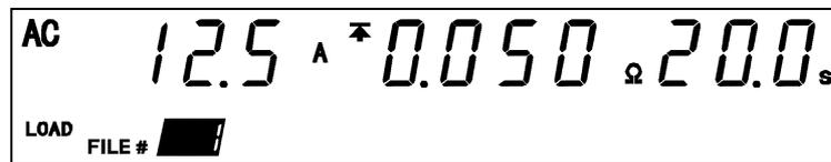
In this status, the preset minimum test valve can be checked by using the **◀** or **▶** key.
