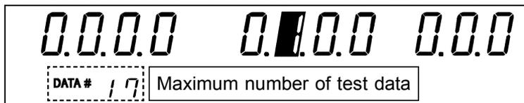
In this example, the maximum number of test data is set at 17. Counting starts at 1 and ends at 17, after which the number reverts to 1.
