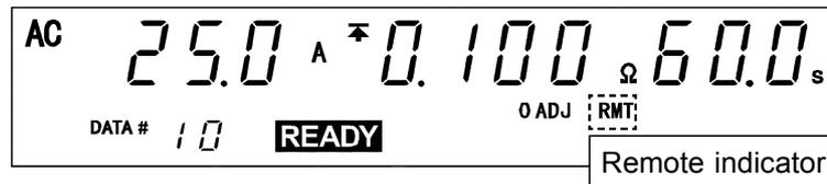
To inactivate the REMOTE state, press **SHIFT** + **0ADJ** (LOCK).
