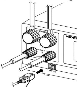
(5) With the 9296 CURRENT PROBE, be sure to connect the probe to the other terminals using the same procedure.
