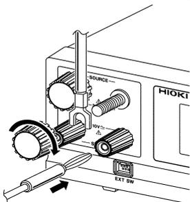
(3) Rotate the current output terminal clockwise to close.
