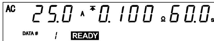
After "Test data count" is set, the output current frequency is replaced by "Number of test data."
