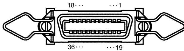
External I/O connector pin numbering
