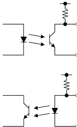
The insulation of the signal lines is for eliminating mutual influences between the signals. Any external device which is connected to the 3157 unit should always be properly protectively grounded. If proper connection to a protective ground is not established, there is a danger of damage to the insulation.
