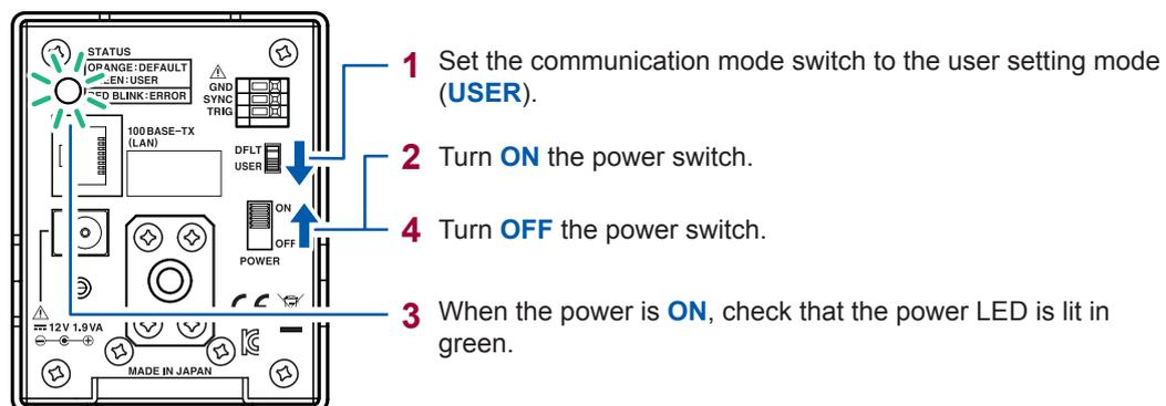
If the power LED is not lit in green, the setting of the communication mode switch may be incorrect or the instrument may malfunction. If the instrument malfunctions, stop the settings and send the instrument for repair.
