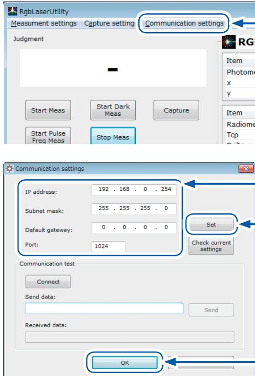
The image shows two screenshots of the RGLaserUtility software. The top screenshot shows the main application window with the 'Communication settings' tab selected. The bottom screenshot shows the 'Communication settings' dialog box with the following fields: IP address (192.168.0.254), Subnet mask (255.255.255.0), Default gateway (0.0.0.0), and Port (1024). The 'Set' button is highlighted, and the 'OK' button is also highlighted.
