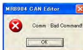
The message to the right will be displayed when the Memory HiCorder is in the process of performing measurement or calculations.
