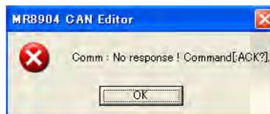
If the message shown to the right is displayed, there may be an illegal value in a definition registered in the register list. Refer to p.26 and p.27 and remove the illegal definition.
