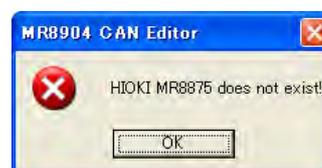
If you click **[OK]** without connecting a Memory HiCorder, the Launch window will be displayed, but the list box on the right of the toolbar will be blank.
