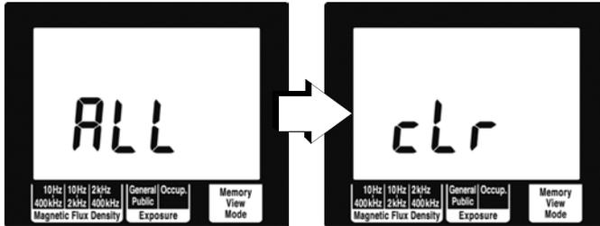
After this it displays the model number and estimated remaining battery life, and is restarted using the factory default settings.
