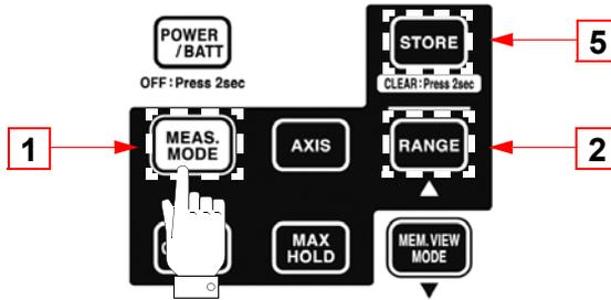
1. Press **MEAS. MODE** to open the exposure level (Occup.) mode screen.
