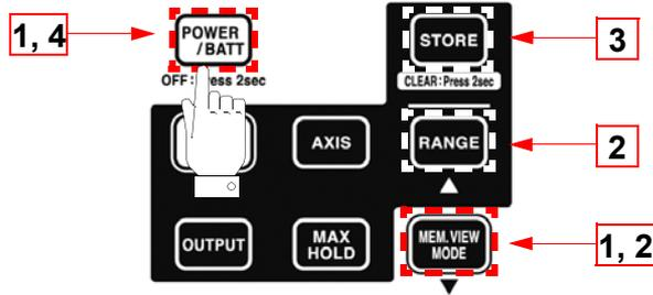
1. When the power is off, hold down **MEM. VIEW MODE** and press **POWER /BATT**.
