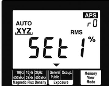
After this follow the procedures 2. (P.48) described in 3.4.3 "Measurement Procedure" to perform an exposure level (General Public) measurement.
