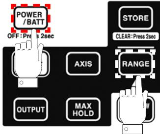
When the power is off, hold down **[RANGE]** and press **[POWER / BATT]**. This deletes all saved measurement data.
