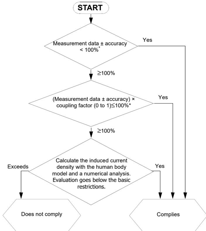
\* : Whether tester accuracy should be added or subtracted depends on the standpoint of testing personnel. Refer to the instructions in the IEC62233 standards. For details on the coupling factor, refer to Appendix 2 "Coupling Factor in the IC-NIRP Guidelines" (P.114).
