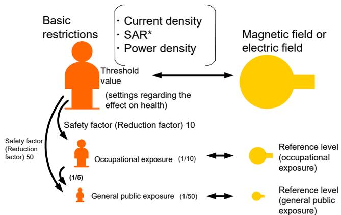
As can be inferred from the above, there is a margin, a safety factor (reduction factor) between the exposure level measured by this tester and the threshold values in the basic restrictions. Thus an exposure level of 100% measured by this tester does not mean to affect the human body.
