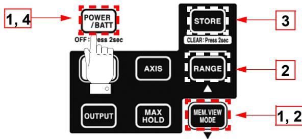
1. When the power is off, hold down **MEM VIEW MODE** and press **POWER / BATT**.
