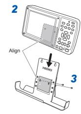
When attaching the LR8410 Wireless Logging Station to the Z1009 Fixed Stand, secure it in place with the included screws from the back.
