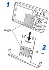
Attach the LR8410 Wireless Logging Station to the holder with the included M3 × 5 mm screws from
