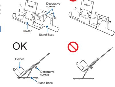
2 Aligning the groove on the holder with the groove on the back of the LR8410 Wireless Logging Station, place the LR8410 on the holder.
