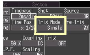
When the trigger mode is set to [Repeat], triggering is disabled during the end of recording processing (auto save, waveform display processing and calculation) before going to the next trigger standby status. Therefore, events that meet the trigger criteria during this processing period are not recognized as trigger events.
