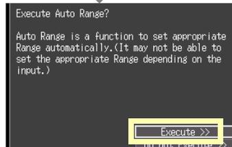
If appropriate settings for the input signal cannot be determined, select [Next] to display the manual range selection procedure, and follow the procedure to make the settings.
