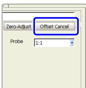
The input value can be forced to display as zero volts. Input signal bias, such as sensor emf, can be adjusted to display as zero volts. This function applies to voltage and current measurement.
