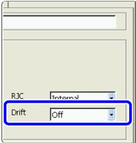
This function periodically corrects for drift of the reference potential (about once per second) to improve thermal characteristics in thermocouple mode.
