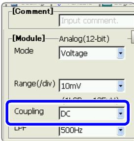
Select the coupling method for input signals
