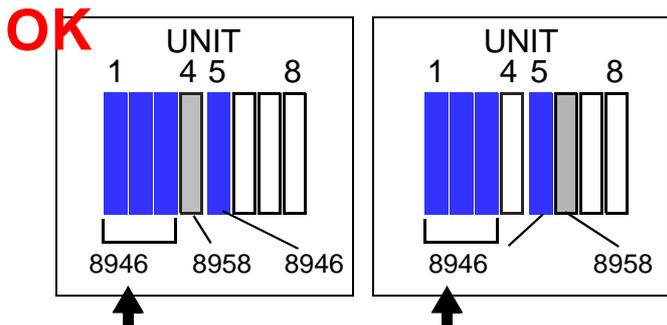
Only a maximum of 3 units of Model 8946 can be installed in the UNIT 1-4 slots.
