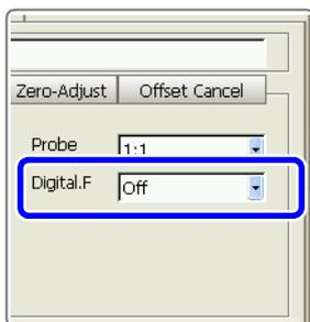
Noise can be removed by applying additional averaging to the measurement data within the input module. With the 8937 Voltage/Temp Unit, digital filtering is available only in the measurement ranges from 500  $\mu$ V to 2 mV/div. The digital filter is not available in other ranges.
