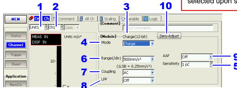
The [Charge] measurement mode is selected upon system reset.
