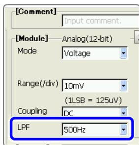
To suppress high-frequency components, select a low-pass filter within the input module
