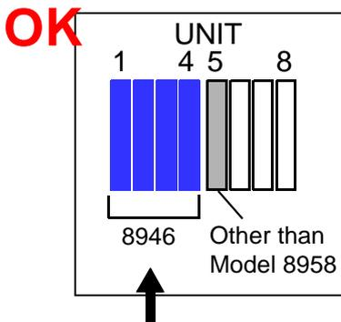
4 units of Model 8946 can be installed to the UNIT 1-4 slots.
