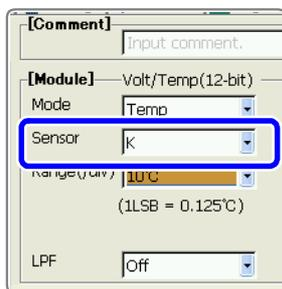
Set to match the type of thermocouple being used.
