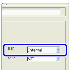
When connecting a thermocouple directly to the input module, select [Internal]. Reference junction compensation is performed within the input module. When connecting through a reference junction device (e.g., a 0°C control tank), select [External].
