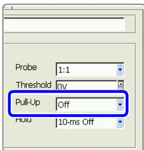
The pull-up resistance function is used when connecting to an open-collector output signal.
