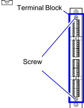
The terminal block can be detached from the Model 8958 16-Ch Scanner Unit.
