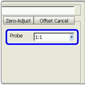
Probe attenuation can be selected when measuring using a connection cable, differential probe or attenuating probe. (Only for voltage measurement)
