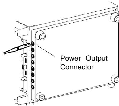
Connect the power cables from the probes to the output connectors of the Model 9687 Probe Power Unit.
