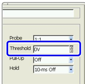
Sets threshold value. Measures when the waveform crosses a preset threshold.
