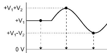
The offset voltage set to display as zero depends on the timing of offset cancellation execution.
