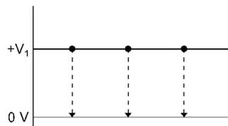
Offset voltage  $+V_1$  is set to display as zero regardless of execution time.
