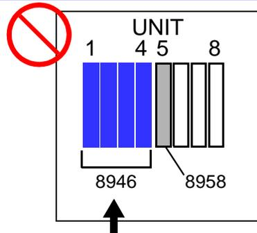
Do not install 4 units of Model 8946 to the UNIT 1-4 slots.
