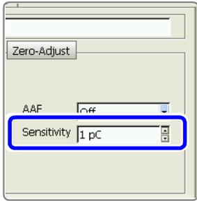
Sets the value per  $m/s^2$  defined for the acceleration sensor to be used.
