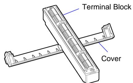
Turn the cover over and place the terminal block on it as shown above for stability while making connections.
