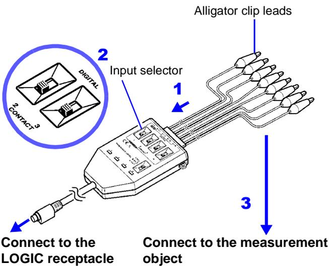
When measuring the contact signal (Contact input)
