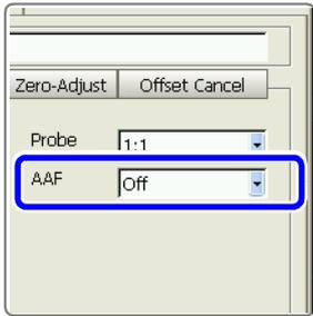
Enable the anti-aliasing filter to remove aliasing distortion. The cutoff frequency is automatically set according to the time axis range setting.
