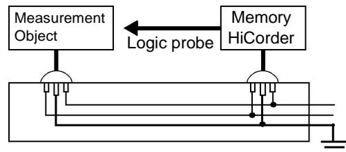
Connect the measurement object's ground to the GND terminal of this instrument. (Always obtain power from the same mains circuit.)
