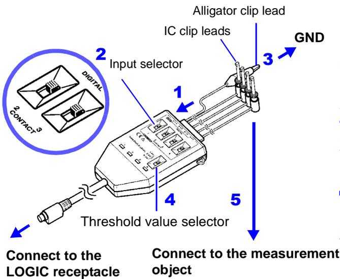
When measuring digital signals (Digital input)
