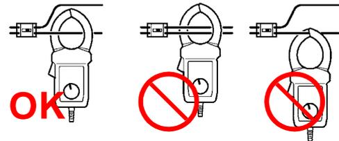
Attach the clamp around only one conductor. Single-phase (2-wire) or three-phase (3-wire) cables clamped together will not produce any reading.
