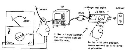
The 9004 Clamp-on Probe which is simply clamped over the line for tests
