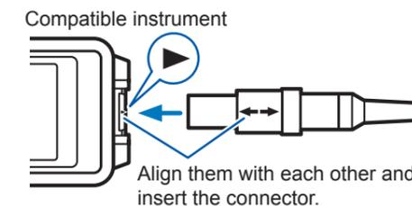
Align the arrow on the device's output connector with the mark ► on the compatible instrument's sensor input connector and insert the connector.
