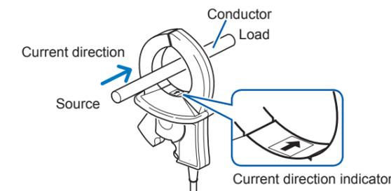
If the clamp is attached with the current direction indicator pointed in the opposite direction of the current, the phase is displayed deviating by 180 degrees.
