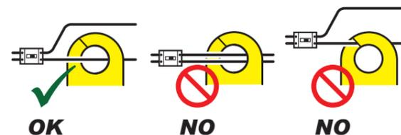
Close the tips of the jaw completely before performing measurement. If the output cable is caught on the jaw or the jaw is forced into the measurement location, it may not close completely. If this occurs, it will not be possible to obtain an accurate measurement.
