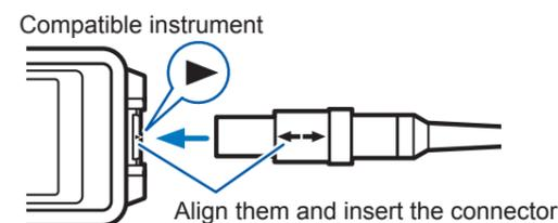
Align the arrow on the device's output connector with the mark ► on the compatible instrument's sensor input connector and insert the connector.
