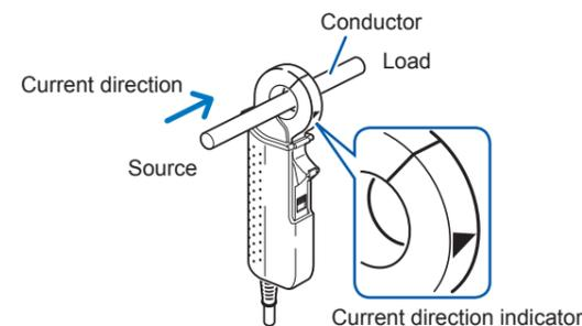
If attached with the current direction indicator pointed in the opposite direction of the current, the phase is displayed deviating by 180 degrees.
