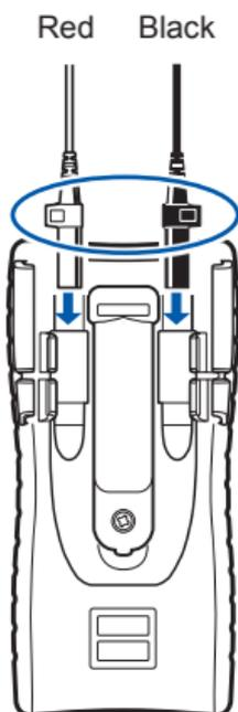
When connecting the test leads to the instrument, push them as far as possible into the measurement terminals while holding the end of the plugs.
