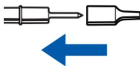
Insert the metal pins of the test leads into the holes of the sleeves, and firmly push them all the way in.
