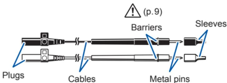
**Metal pin** Connect to the object to be measured.
