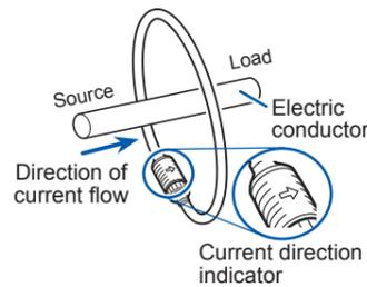
Clamp only the conductor you wish to measure with the current direction indicator pointing toward the load side. (To ensure that the measured current and sensor output have the same phase.)
