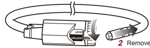
1 Rotate the dial until the blue ◀ mark is in the **UNLOCK** position.
