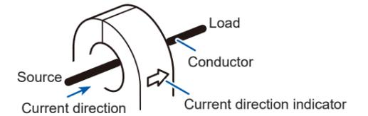
Gripping the lever to open the jaw, align the current direction indicator with the direction of the current in the conductor, and close the jaw with the conductor roughly centered in the jaw.
