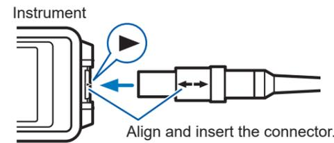
Align the arrow on the device's output connector with the ► on the compatible instrument's sensor input connector and insert the connector.
