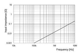
Fig.5 Input impedance (Typical) (3274)
