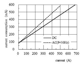
Current consumption\* vs. current to be measured (typical)(3275) \*The sum total of a positive and negative current consumption
