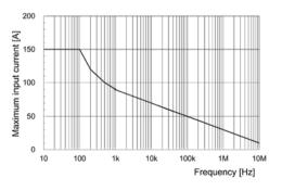
Fig.3 Derating according to frequency(3274)
