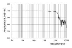
Fig.1 Frequency characteristics (Typical) (3274)
