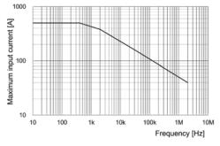
Fig.4 Derating according to frequency(3275)
