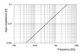
Fig.6 Input impedance (Typical) (3275)
