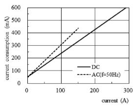
Fig.7 Current consumption\* vs. current to be measured (typical)(3274) \*The sum total of a positive and negative current consumption
