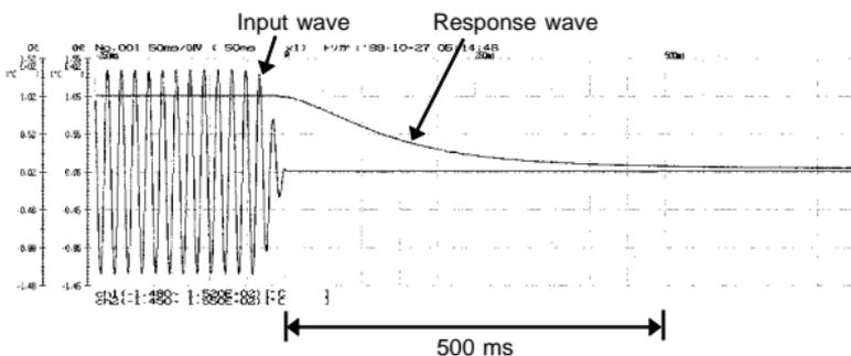
Fig. 2 Waveform of Measurement Response (Fall)
