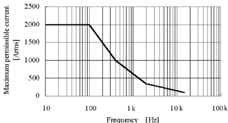
Fig.3 Frequency-dependent deletion characteristics
