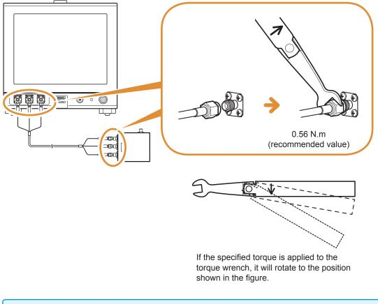
Do not rotate the cable when connecting the SMA connector of the cable to the instrument and the test head. If the cable is rotated while connecting the connector, the core wires of connector or cable may get damaged. Rotate the nut of the connector and connect.
