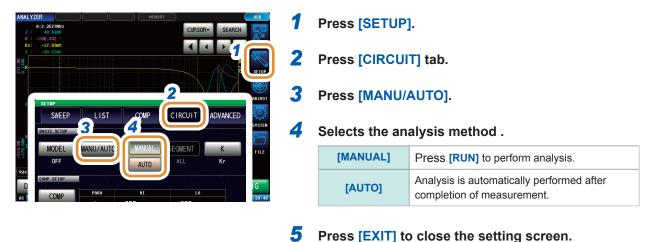
Equivalent circuit analysis cannot be performed with [MANUAL] in the continuous measurement screen. To perform equivalent circuit analysis during continuous measurement, change the setting to [AUTO] and save the panel.
