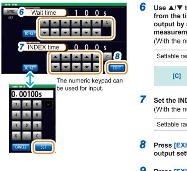
Use ▲/▼ to set the wait time (time to stabilize) from the time a measurement signal has been output by applying a trigger to the start of the next measurement.
