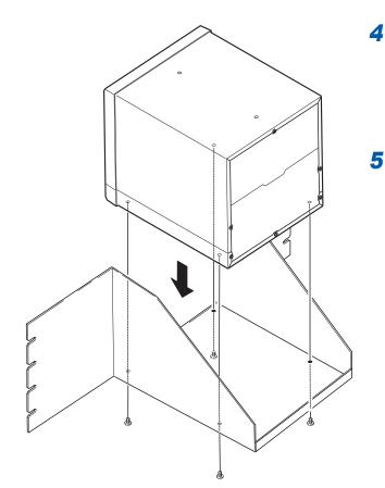
Install the spacers on both sides of the instrument, affix the rack mounting plate with the screws removed from the legs (M3 × 10 mm).
