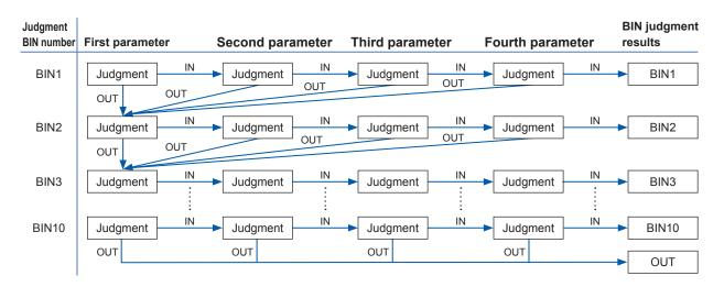
The measurement elements can be ranked by setting a series of severe to lenient judgment standards as shown in the following diagram.
