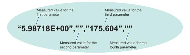
The above shows that the first parameter is "5.98718  $\Omega$ ", the third parameter is "175.604°". Measured values for the second and fourth parameters are not displayed as they are OFF.
