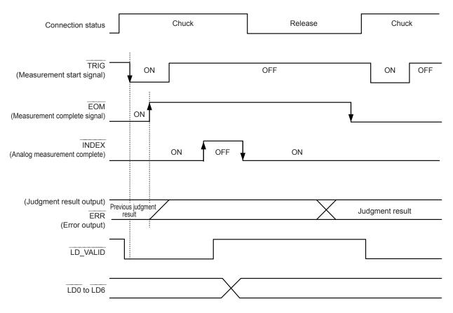
EOM:OFF From trigger to the end of measurement INDEX:OFF Probe chuck period (Do not disengage the probe.)
