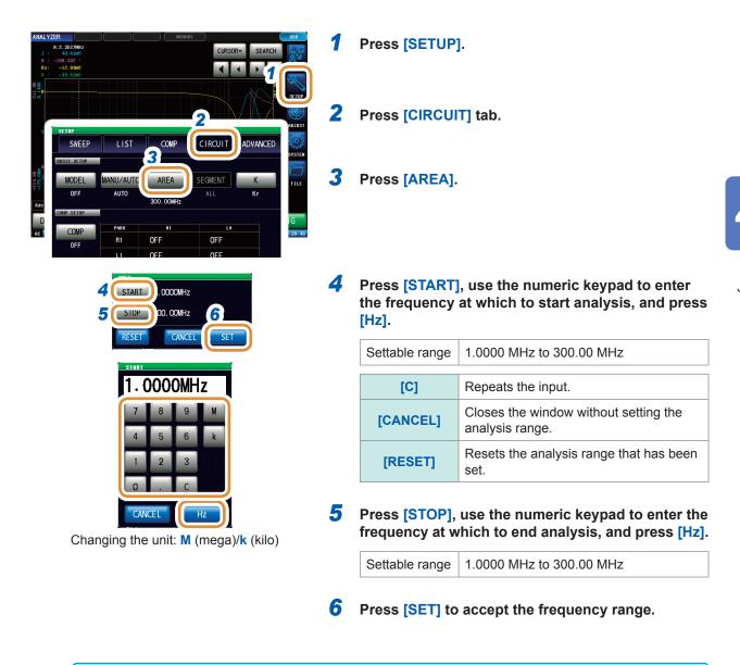
The accuracy of the analysis may deteriorate if a very narrow frequency range is set.
