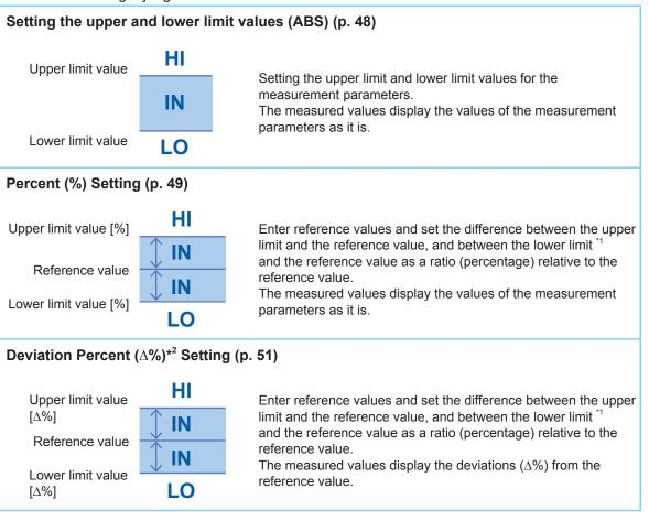
\*1 The following formula is used to calculate the comparison upper limit value and comparison lower limit value. (For the comparison lower limit value, if a value that is lower compared to the reference value is set, a minus (-) sign is required for the percentage setting value.)
