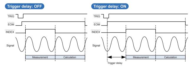
While trigger delay is being used, the LED for indicating that measurement is in progress is lit.
