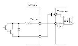
Connection with PLC output (positive common output)
