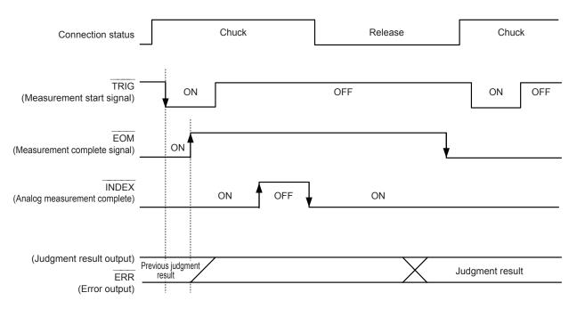
EOM:OFF From trigger to the end of measurement INDEX:OFF Probe chuck period (Do not disengage the probe.)
