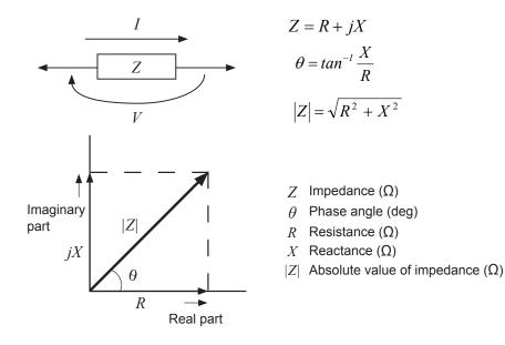
In addition, admittance Y, the reciprocal of impedance Z can also be used depending on the characteristics of the circuit components. The following values can also be determined from admittance Y by mapping admittance Y to the complex plane in the same way as impedance Z.
