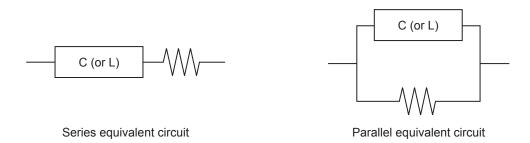
Measurement values of both modes can be displayed because measurement value in each equivalent circuit mode is obtained by calculation. However, please note that the appropriate equivalent circuit depends on the test sample.
