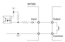
Connection with PLC output (negative common output)
