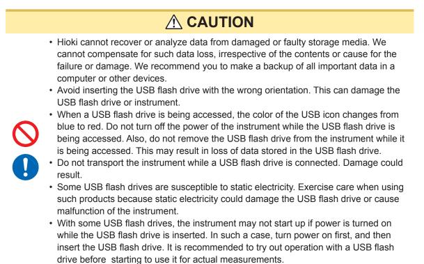
USB flash drives have limited usable lifetime. Data reading and writing will fail after long-term use. Replace the USB flash drive in this case.
