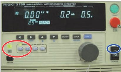
Check that **no one is near the testing area**, and turn on the main power switch of the 3159.
