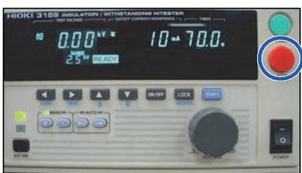
Press the STOP (EXIT) key to confirm the test conditions. The 3159 enters the READY state. (The figure on the left shows the 3159 when the test conditions have been confirmed.)
