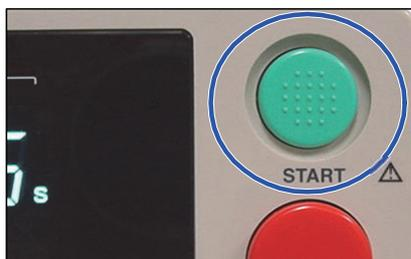
Press the START key to start the test.
