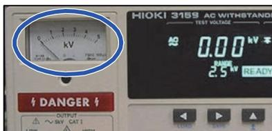
Check that the analog voltmeter is indicating **0 kV**
