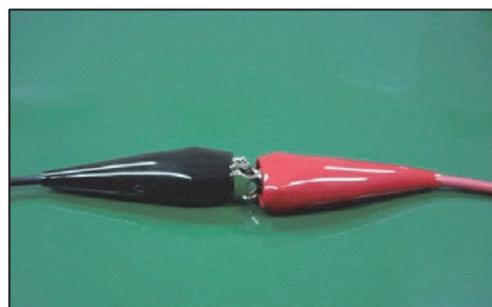
Short-circuit the high-voltage test lead (red) and low-voltage test lead (black) as shown in the picture.
