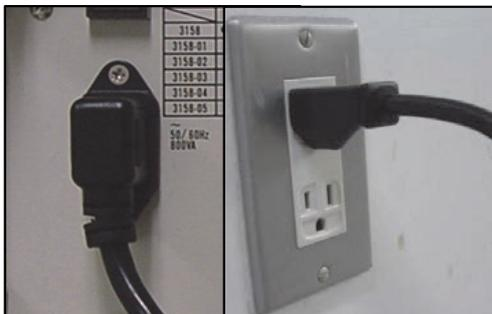
Connect the **power cord** (supplied with the 3159) to the inlet of the main unit and a **grounded outlet**.
