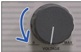
Return the output voltage knob to **zero**. (Turn the knob all the way counter-clockwise)
