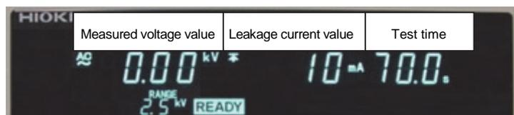
Set the three parameters mentioned in "1. Preparation": **Test voltage**, **Reference leakage current value** (upper limit for the test), and **Test time**. Refer to "3. Simple Startup Inspection (Settings)."
