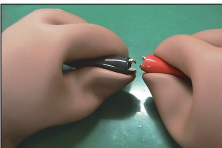
Disconnect the test leads (short-circuited part).
