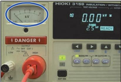
Check that the analog voltmeter indicates **0 kV** and that the
