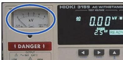
Check that the analog voltmeter is indicating **0 kV**
