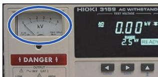
Check that the analog voltmeter indicates **0 kV** and that the **DANGER** lamp is **not illuminated**.
