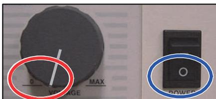
Turn the output voltage knob all the way counter-clockwise, returning it to **zero**. Turn the main power switch of the 3159 off.
