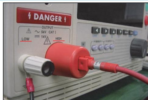
Tightly attach the supplied **low-voltage test lead** (black) to the **LOW** terminal (black).
