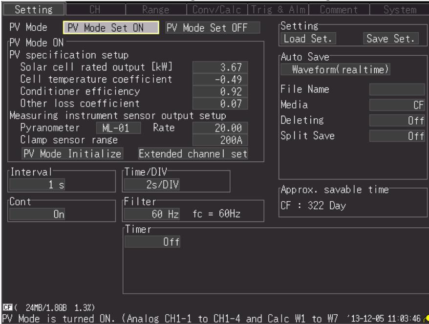
Note: The version of the software until the V9.12, it was ML-020 only rather than selection of pyranometer kind. From V9.13, please use it to select "ML-01", "ML-020", and "Free Set" pyranometer kind used as shown in the figure on the left. (In the system screen, you can check the version.)
