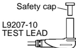
1. Remove the protective cap from the test lead supplied with the product.
