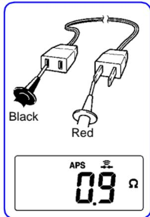
3. Connect the test leads to the measurement object.
