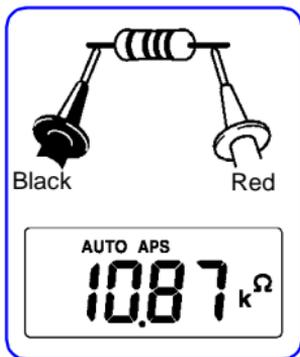
2. Connect the test leads to the measurement object, and read the indicated value.
