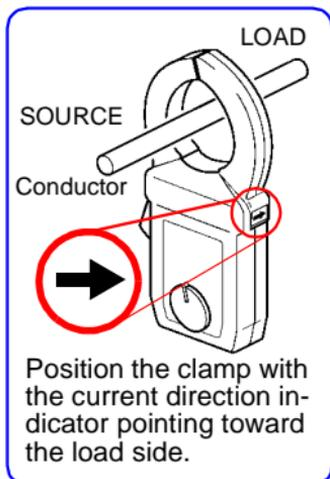
Make sure the range setting of the product is the same as that of the Clamp-on probe before starting measurement.
