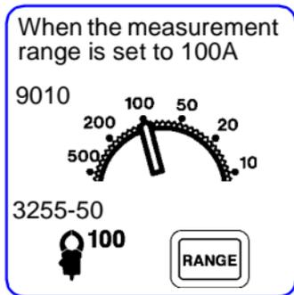
2. Set the measurement range of the Clamp-on probe (option).
