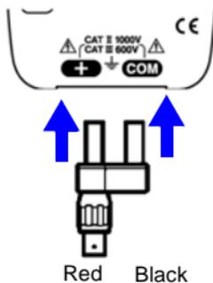
Connect the red plug of the Conversion adapter to terminal **+**, and the black plug to terminal **COM**.
