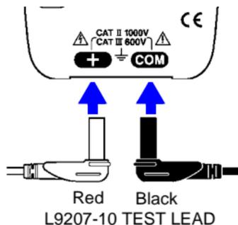
2. Connect the red test lead to terminal +, and the black test lead to terminal **COM**.
