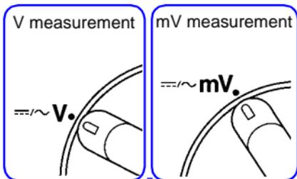
1. Move the function selector to the **V** or **mV** position ("V" or "mV" lights up,  $\sim$  lights up).
