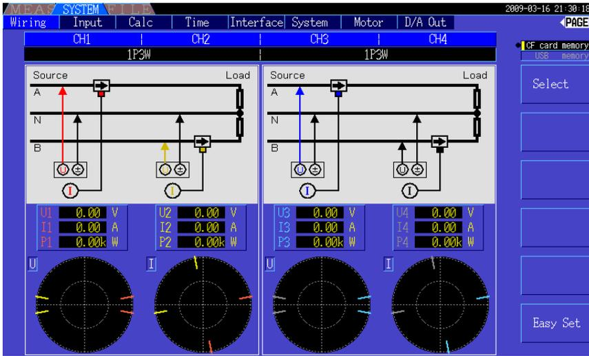
Wiring Mode 5. 3-phase, 3-wire (3P3W2M) + single-phase, 3-wire (1P3W)
