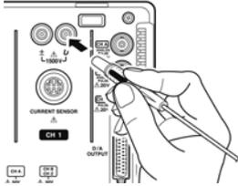
Plug the voltage cables into the appropriate channels' voltage measurement jacks. Insert the plugs into the terminals as far as they will go.
