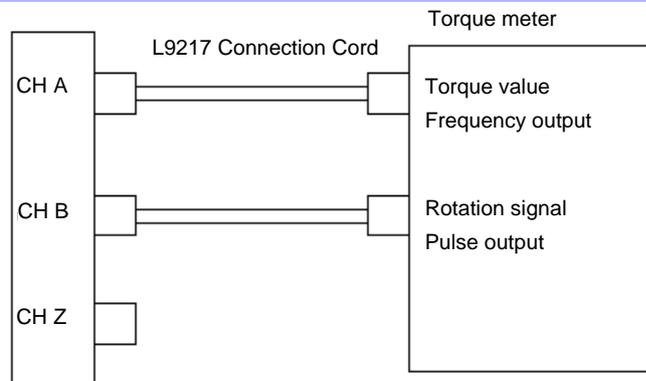
**Example 3. Connecting the torque meter that provides torque values and the incremental rotary encoder**
