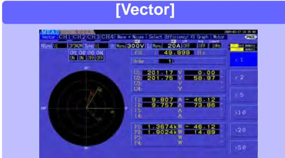
This page displays measured voltage, current, and power on channels 1 to 4 as numerical values and as vectors.
