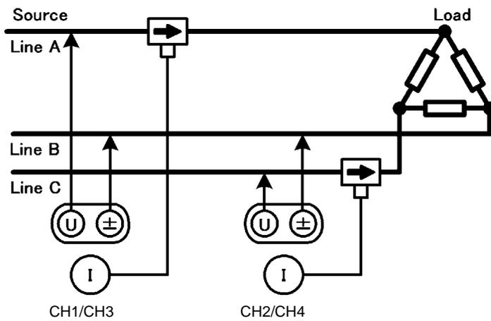
3-Phase, 3-Wire, 3-Measurement (3P3W3M)
