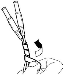
2. Wind the spiral tube around the leads.
