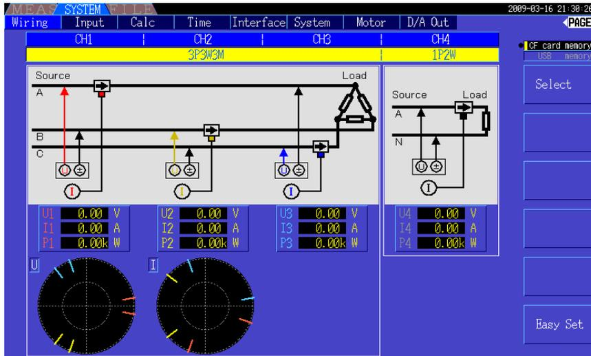
Wiring Mode 8. 3-phase, 4-wire (3P4W3M) + single-phase, 2-wire (1P2W)
