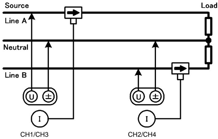
3-Phase, 3-Wire, 2-Measurement (3P3W2M)
