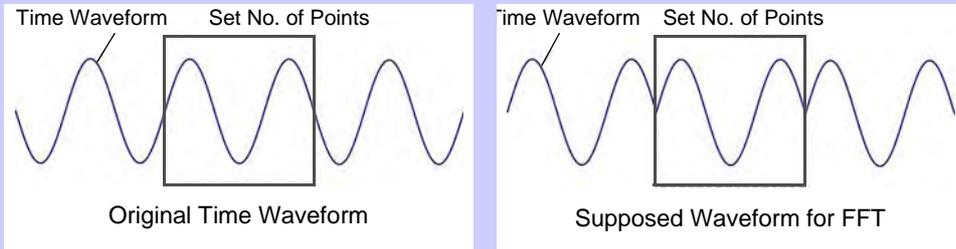
When the number of points specified for FFT calculation does not coincide with the measurement waveform period, the edges of the waveform within the window become discontinuous (called "leakage errors"), and non-existent noise is detected. The Window type provide means of suppressing leakage errors by smoothly connecting the edges of the waveforms.
