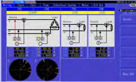
Select the appropriate wiring mode (phase system configurations) and execute quick setup on this page. Wiring diagrams for each mode depict the appropriate measurement cable connections.
