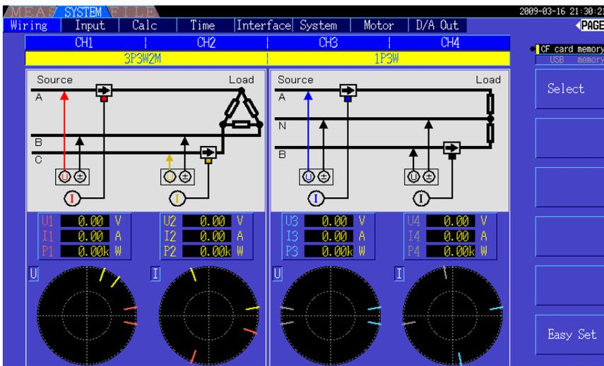
Wiring Mode 6. 3-phase, 3-wire (3P3W2M) × 2
