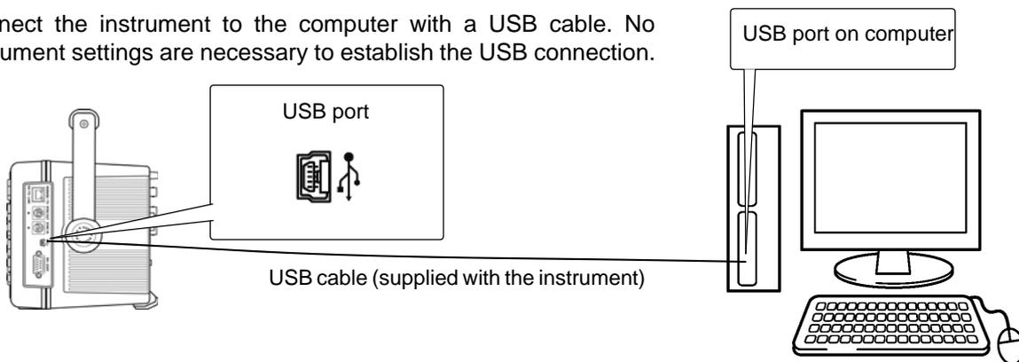
The USB indicator is displayed when the connection to the computer is established.
