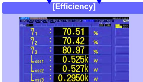
This page displays the numerical values of efficiency and loss determined by calculation formulas.
