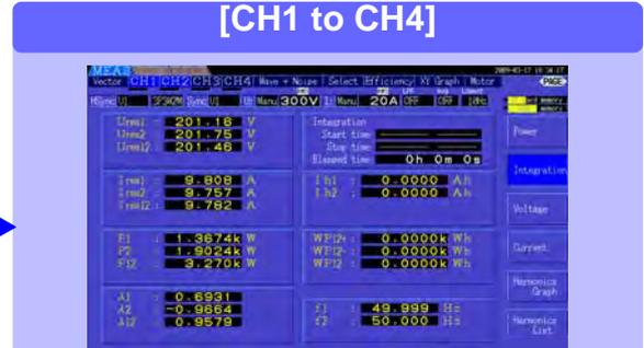
This page displays measured power, voltage and current values, integration values, and provides access to harmonic graphs and lists for each channel.
