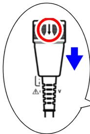
With the arrow on top of the plug, plug each current sensor cable into the appropriate channel's current measurement jack. Insert each plug until you hear it lock.
