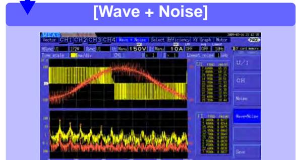
This page displays voltage, current, and noise waveforms. The waveforms can be saved.
