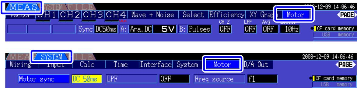
The motor analysis function acquires signals from rotation-sensing devices such as a torque sensor and rotary encoder and measures motor analysis items (torque, rotation rate, motor power and slip). Motor efficiency, total efficiency and loss can be calculated when combined with the "4.7 Viewing Efficiency and Loss Measurement Values" (p. 78) functions.
