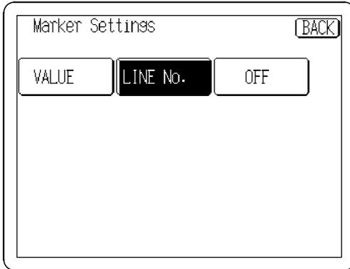
Press the **LINE No.** button on the Marker Settings screen so that it displays in reverse.
