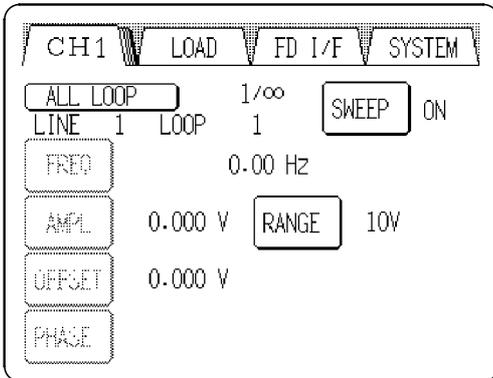
1. Press the **BACK** button with sweep ON in Section 3.7.16 to return to the Output setting screen (see Section 2.5). The **ALL LOOP** button appears on the upper left of the Output setting screen.
