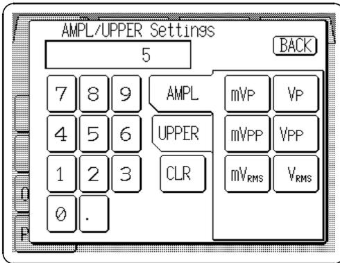
7. Press the Amplitude/Upper limit setting button (**AMPL/UPPER**) on the Output setting screen, and the AMPL/UPPER (amplitude/upper limit) Settings window appears.
