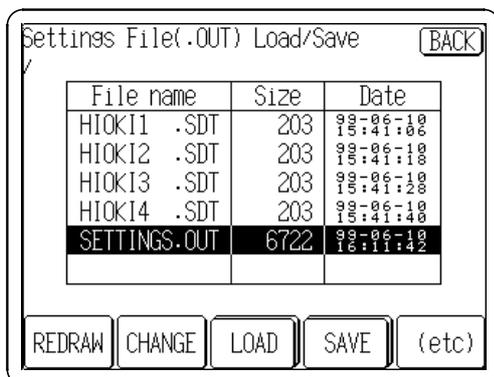
1. Insert the floppy disk and press "File Utility" on the FD I/F screen. If the **LOAD** button is not displayed, press (etc) to display the **LOAD** button.
