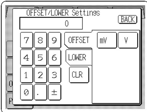
9. Press the Offset/lower limit setting button (**OFFSET/LOWER**) on the Output setting screen, and the OFFSET/LOWER (lower limit) Settings window appears.
