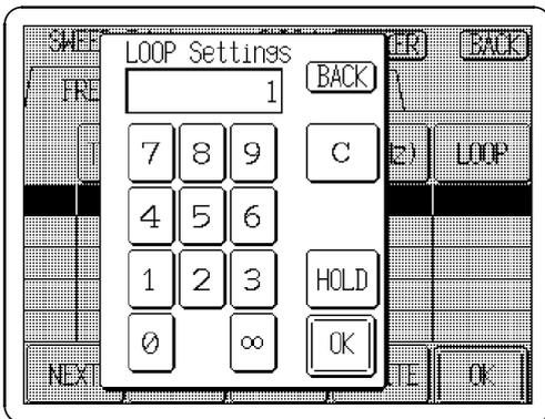
1. Press the **LOOP** button to open the LOOP Settings window.
