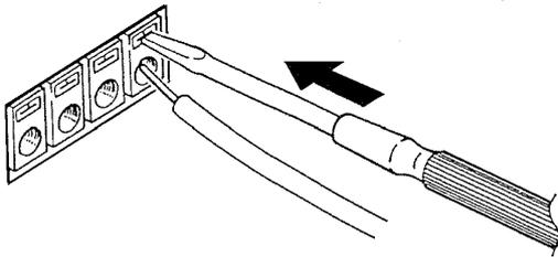
1. Use suitable wires bared at their ends for a length of about 10 mm.
