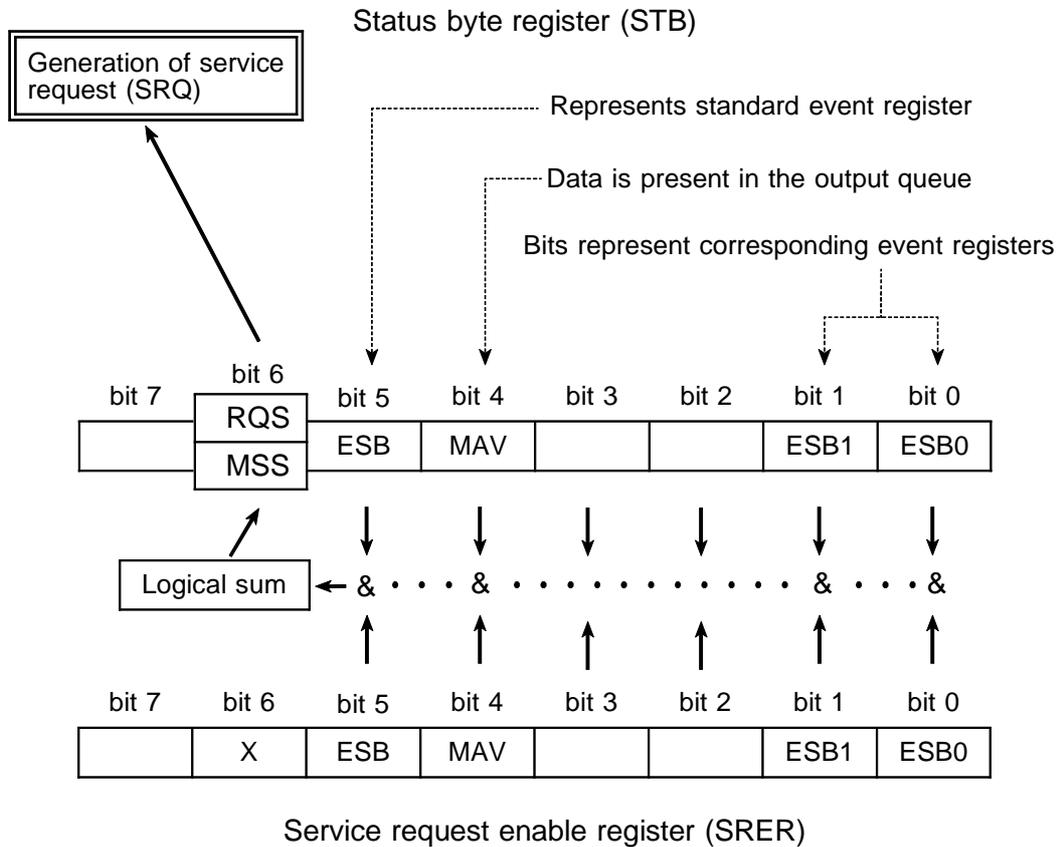
The status byte register holds information relating to the event registers and the output queue. It is further possible to use the service request enable register as a mask to select the items required. If any of the bits selected by the mask becomes 1, bit 6 (the master summary status or MSS bit) is also set to 1, an RQS message is generated, and this generates a service request.
