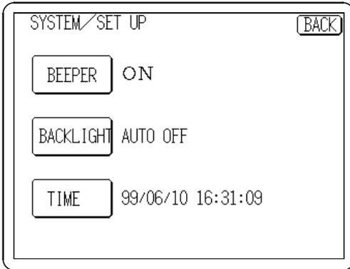
This screen is for miscellaneous settings. The beeper, automatic backlight off and time can be set.
