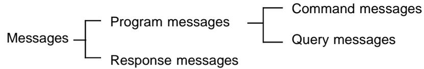
Of these, program messages are those received by the unit from the controller, while response messages are those sent from the unit to the controller. During addressable, program messages are those received by the unit from the external controller, while response messages are those sent from the unit to the controller.
