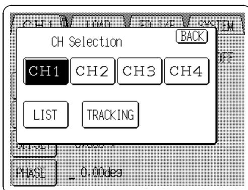
1. Pressing a tab to display channel numbers opens the CH Selection window.
