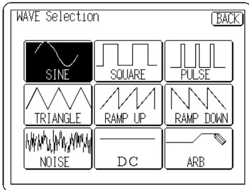
1. Press the Waveform display button on the Output setting screen, and the WAVE Selection screen appears.
