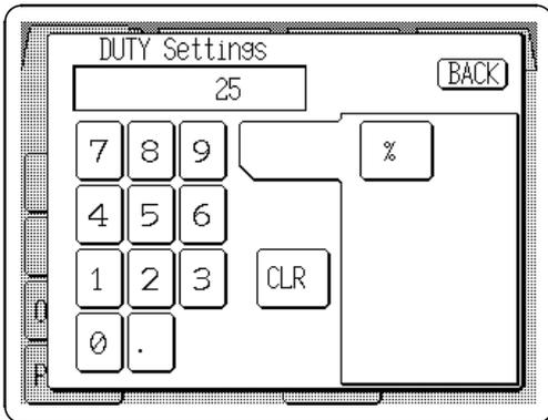
1. Press the Duty setting button (**DUTY**) to open the DUTY Settings window.
