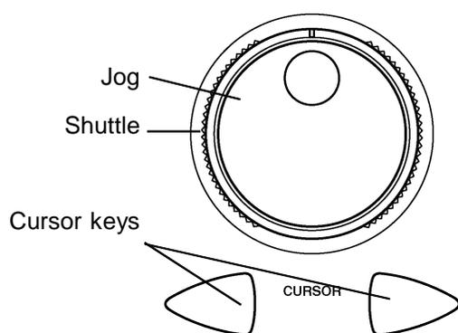
The Jog and Shuttle controls are used in combination with the cursor keys to set and change values.
