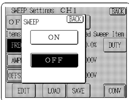
1. Press the Sweep setting button on the Sweep Settings screen to open the **Sweep ON/OFF** switching window.
