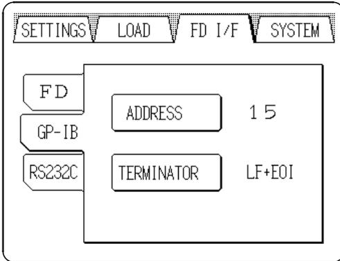
The GP-IB setting is used when the 7075 is to be controlled remotely by GP-IB.
