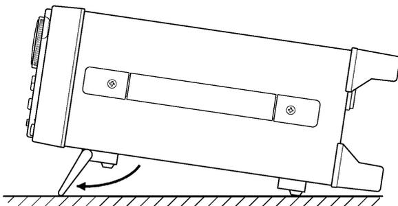
The unit should be placed either level, or tilted using the bail.
