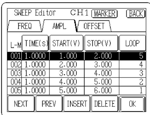
Press the **MARKER** button on the SWEEP Editor screen (see Section 3.7.6, "Selecting the Sweep Editor Screen") to display the Marker Settings screen.
