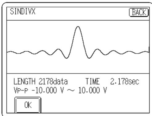
The information of waveform size, output time, and amplitude for the specified waveform is displayed.
