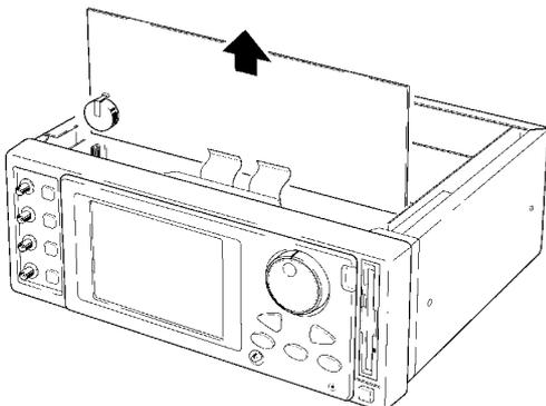
4. Remove the front-most board (MPU board), on which the lithium battery is installed.
