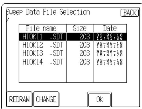
Sweep settings that have been saved to floppy disk can be loaded back into the unit:
