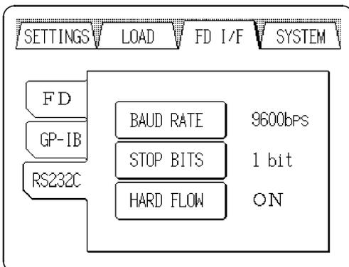
Set the baud rate, stop bit, and hardflow on the RS232C screen.
