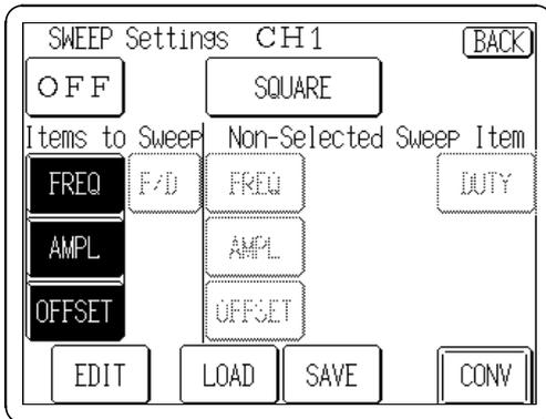
Press the **FREQ**, **AMPL** or **OFFSET** buttons so that the items to be swept are displayed in reverse.
