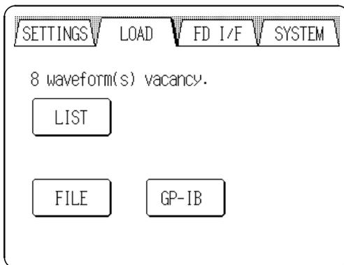
Pressing the "**LOAD**" tab at the upper left of the screen causes the Waveform Input screen to appear.
