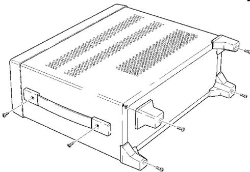
1. Remove the screws in the four support feet on the rear of the unit.
