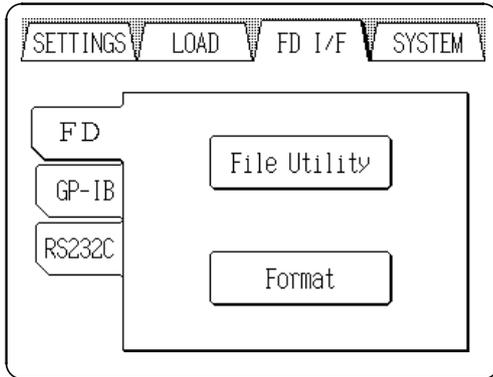
Settings can be saved to and later reloaded from a floppy disk. Files can also be deleted and directories created. The floppy drive uses MS-DOS\* formatting.
