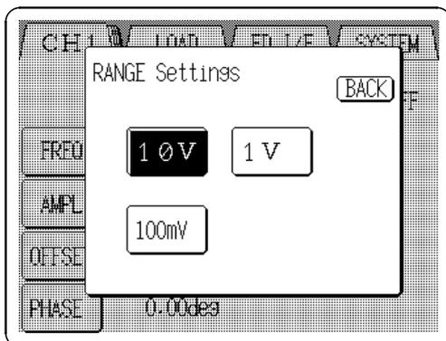
5. Press the Range setting button on the Output setting screen, and the Range setting window appears.
