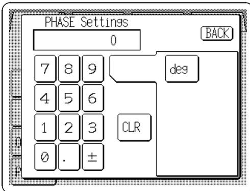
11. Press the Phase/delay setting button (**PHASE/ DELAY**) on the Output setting screen, and the PHASE Settings window appears.
