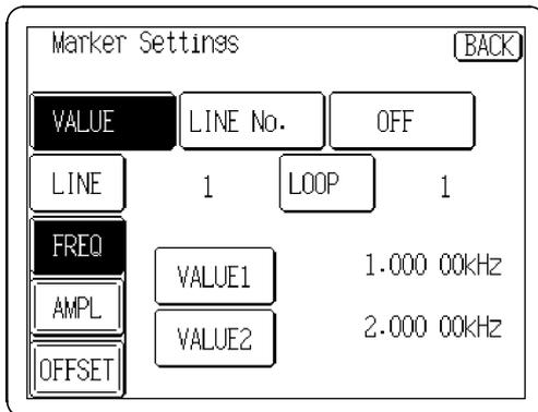
Press the **VALUE** button on the Marker Settings screen so that it displays in reverse. The screen shown on the left is displayed.
