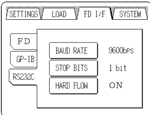
The RS-232C setting is used to transfer waveform data from the 7990 WAVEFORM CREATION SOFTWARE via the RS-232C interface.
