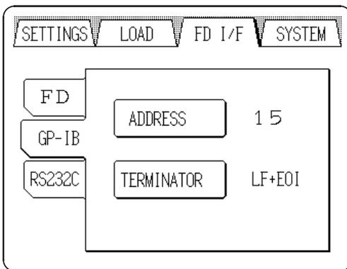
Set the function, address, transmit terminator on the GP-IB screen.
