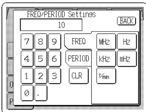
3. Press the Frequency/Period setting button (**FREQ/PERIOD**) on the Output setting screen, and the FREQ/PERIOD Settings window appears.
