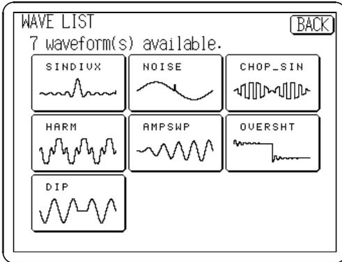
1. Press the **LIST** button, and the input waveform list is displayed.
