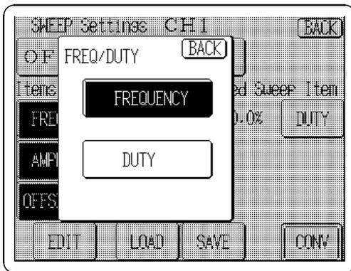
The frequency or duty cycle of pulse waveforms can be swept.
