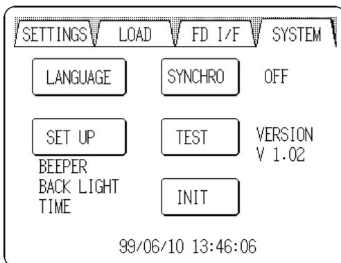
Pressing the **SYSTEM** tab at the upper right of the screen causes the SYSTEM screen to appear.
