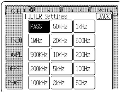
Select the cut-off frequency of the low pass filter.
