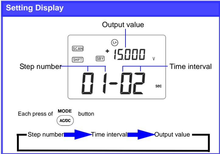
3. Press the [MODE] button to select the step number, time interval or output value. The parameter digit to be set blinks.
