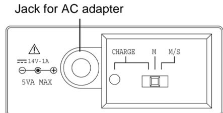
3. Verify that the mains voltage matches the input voltage of the AC adapter, and plug the adapter into an outlet.
