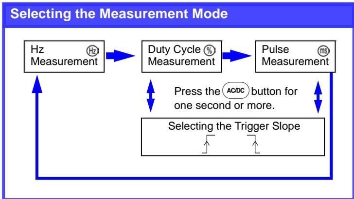
4. Hold the [Hz] button for one second to return to the status in Step 1.
