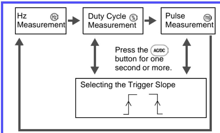
4. Hold the [Hz] button for one second to return to the status in Step 1.
