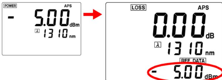
The measurement mode changes from optical power to optical loss and the measurement reading becomes approximately 0.00 dB. (It may not show exactly 0.00 dB depending on the stability of the light source for measurement or connection condition of the reference cable.) A reference value is stored for every wavelength.
