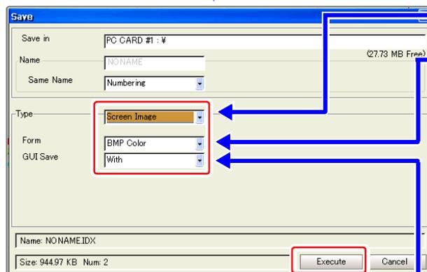
Use the **CURSOR** keys to move the cursor to the setting item, and select the desired setting contents with the **F1** to **F8** key.
