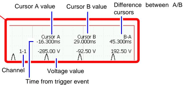
To remove the cursors, press the **FUNCTION** key to return to the FN mode, and press the **F1 [Switch Info]** key.
