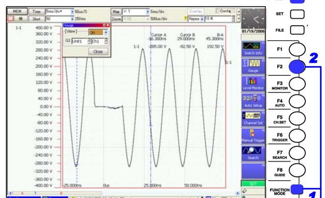
To change the gauge of a displayed channel, press the **FUNCTION MODE** key to enable the FN mode, and press the **F2 [Gauge]** key. In the dialog, select the channel for which to display the gauge.
