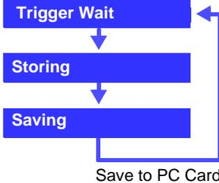
The instrument's measurement status is displayed on the Status bar.
