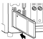
Insert a PC Card into PC CARD Slot 1.
