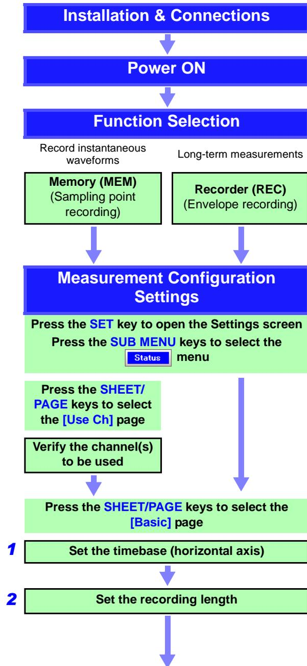
**Install the input modules and cables required for measurement ( $\Rightarrow$  p. 37).**
