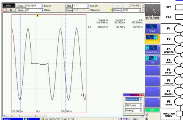
Press the **DISP** key to display method. (Waveform/ Waveform and Information Display/ Gauge and Waveform Display/ Gauge, Waveform and Information Display)
