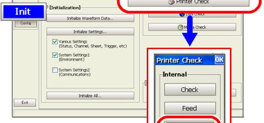
Use the **CURSOR** keys to move the cursor to the **[Printer Check]** button, and press the **F1 [Execute]** key.
