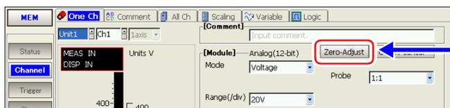
**Execute zero-adjust 30 minutes after turning power on.**
