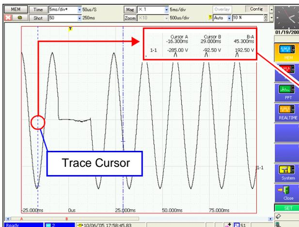
Turn inner knob A or outer knob B to move the cursor to the point to be read.
