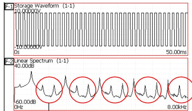
Non-existent frequency components are observed.
