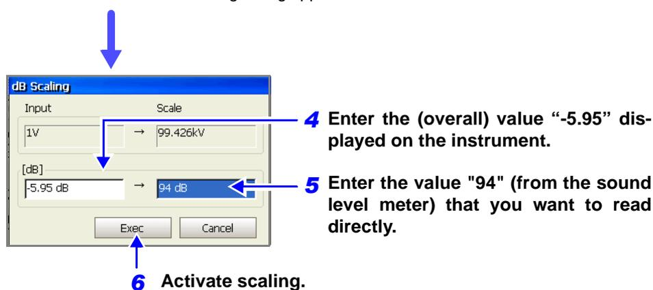
Scaling is performed automatically, and the corresponding values appear in the conversion ratio fields.
