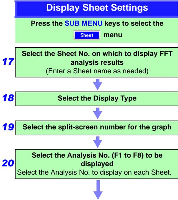
(Configure the Waveform screen display layout)
