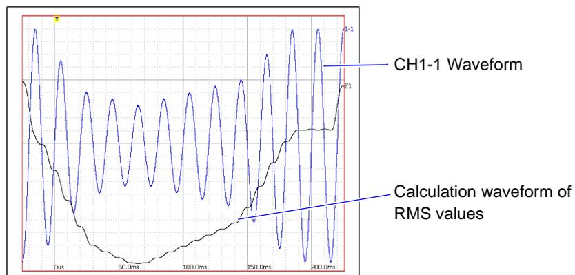
To view the waveform calculated from the acquired data, press the [Execute] button on the Waveform Calculation Settings screen.
