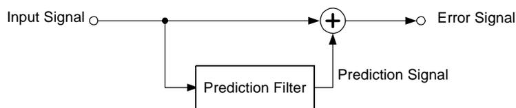
Given a time-discrete signal  $\{x_t\}$  ( $t$  is an integer) where the input signal is sampled at interval  $\Delta T$ , LPC analysis presumes the following relationship between current sample value  $x_t$  and the value of previous sample  $p$ .
