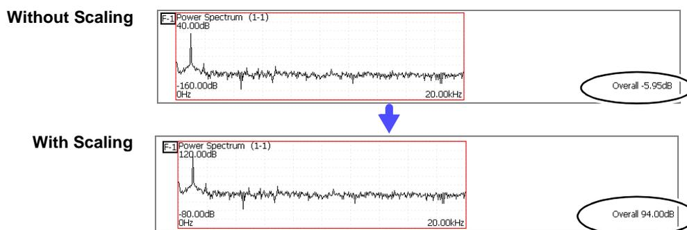
Setting example: To display measurement data on this instrument so that it corresponds to that on a sound level meter.
