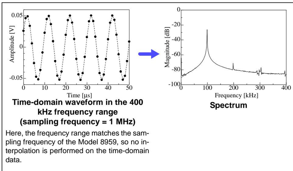
To avoid imaging phenomena when analyzing waveforms with the FFT function, verify the maximum sampling frequency of the input module before measuring.
