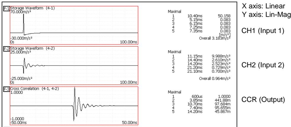
This instrument provides a circular cross-correlation function. Analysis results are normalized to the maximum value.
