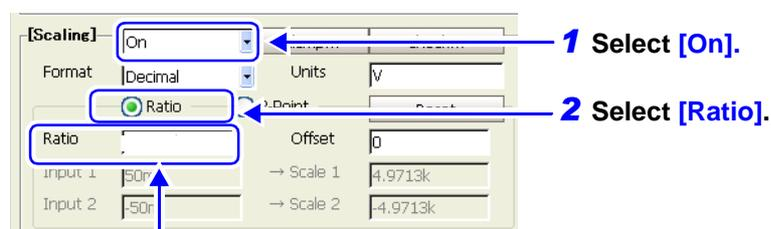
**3** Move the cursor to [Ratio], and press the **F7 [dB]** key.
