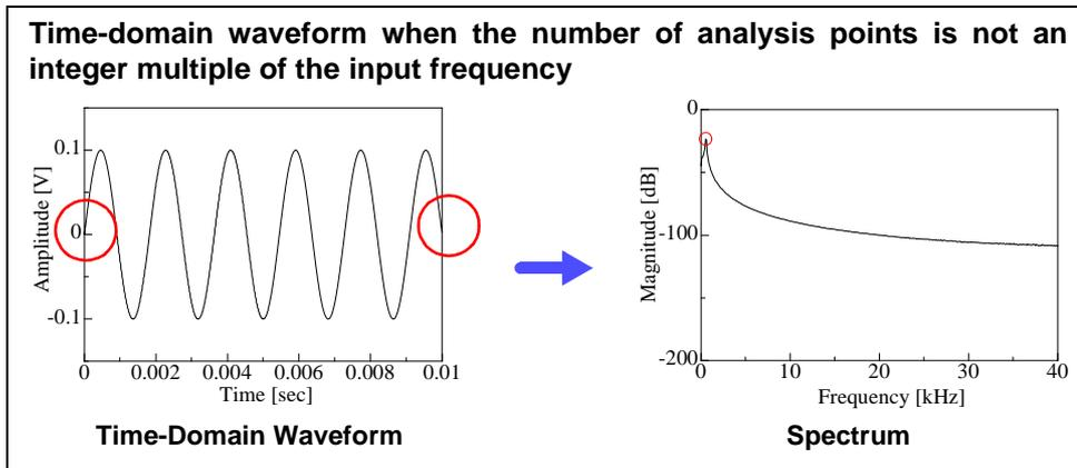
The window function was created to suppress such leakage errors. The window function smoothly connects each end of the time-domain waveform where it is cut off.
