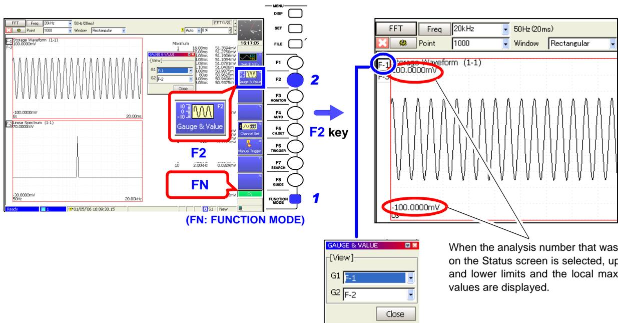
When the analysis number that was set on the Status screen is selected, upper and lower limits and the local maxima values are displayed.
