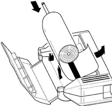
3. Insert the leading edge of the recording paper from bottom into the gap behind the printer roller, and pull it out to the other side. Pressing the FEED key feeds paper.
