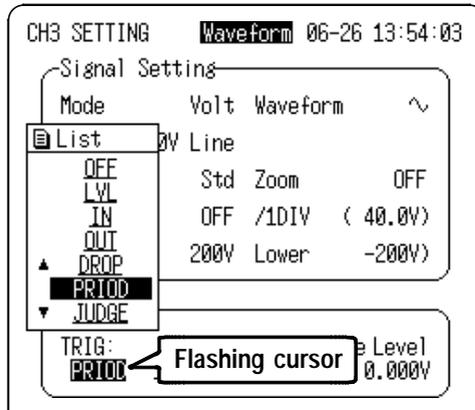
3. Move the flashing cursor to the position shown in the figure below, and set the lower limit of the trigger level (period range) using the ▲/▼ keys.
