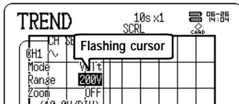
Pressing the RANGE key moves the flashing cursor automatically to the Time Axis position for setting.
