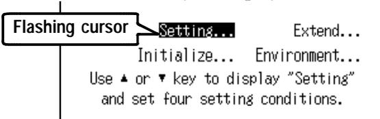
2. Move the flashing cursor to Setting... and use the ▲/▼ keys to display the Setting screen.
