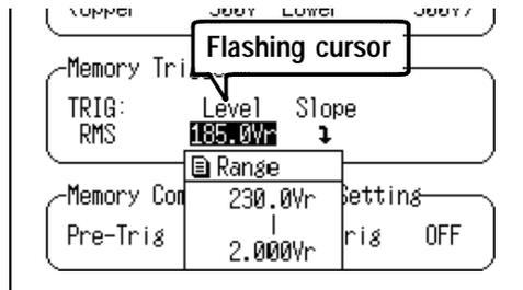
4. Move the flashing cursor to the position shown in the figure below, and set the trigger slope using the ▲/▼ keys.
