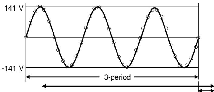
Sample the 50 Hz or 60 Hz waveforms at  $250 \mu\text{s}$  and calculate one RMS value item using three-period data.  $1/800\text{seconds}$
