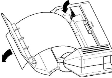
5. Pull the end of the recording paper out at least 10 cm, and make sure that it is positioned quite straight.
