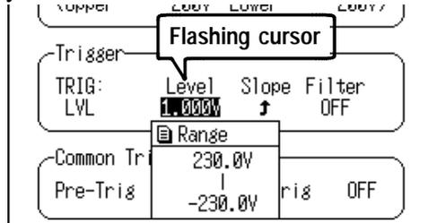
4. Move the flashing cursor to the position shown in the figure below, and set the trigger slope using the ▲/▼ keys.
