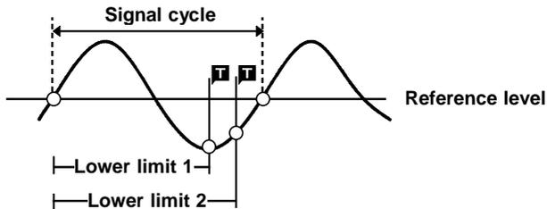
When the upper limit of the set period range appears on the screen before the signal crosses the reference level at the set trigger slope, the upper limit is defined as the triggering position. The triggering position is determined by the position of the upper limit in the period range, as shown in the figure above.
