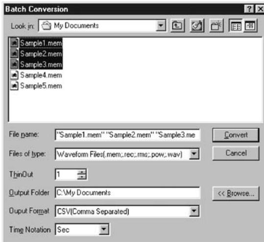
3. If required, specify the sampling intervals in the [**ThinOut**] box at which data is to be converted. Remember that not all data needs to be converted. This setting is useful when you need data over a broad time span.
