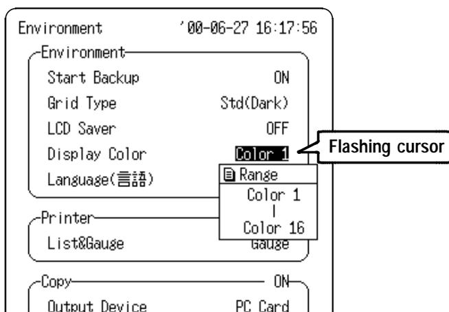
When colors 1 to 6 are selected, the screen displays are shown in colors. The settable items are displayed in yellow, and non-settable items are displayed in gray. When colors 7 to 16 are selected, the screen displays are shown in single color. Settable items are underlined (    ) and non-settable items are displayed as double lines(    ).
