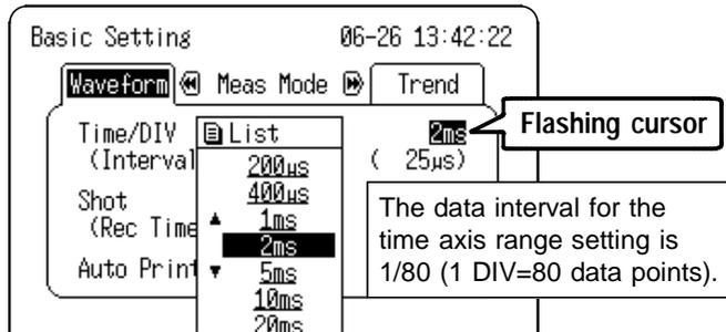
Pressing the TIME/DIV key moves the flashing cursor automatically to the Time Axis position for setting.
