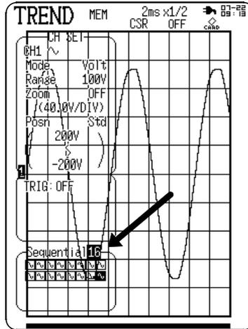
Press CH1 to CH4 on the Instantaneous Recording screen (MEM) to move the flashing cursor to the Sequential position or directly to the frame (  ) where the waveform is recorded.
