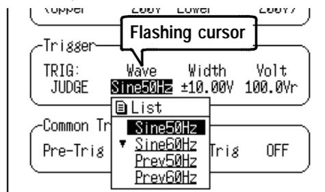
4. Move the flashing cursor to the position shown in the figure below and set the control range using the ▲/▼ keys.
