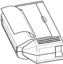
8. Close the stock cover, and finish by tearing off the recording paper against the edge of the printer exit slot.
