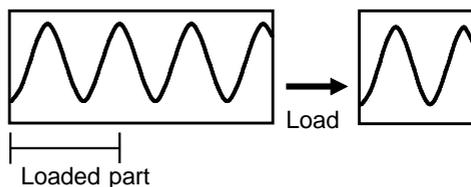
If the recording length set in the 8715-01 is longer than the saved data, the data from the end of the last saved waveform to the end of the 8715-01 recording length is invalid.
