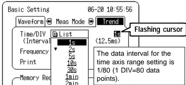
Pressing the TIME/DIV key moves the flashing cursor automatically to the Time Axis position for setting.
