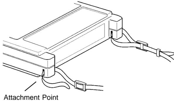
2. Thread the end of the strap through the buckle twice as shown below.
