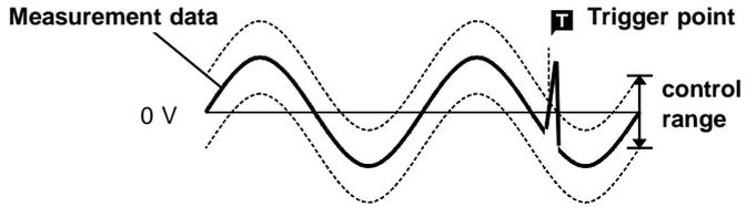
For purposes of creating a control range for a standard waveform (either a sine wave or the previous cycle), one cycle period is considered to begin at the positive-going 0-volt crossing (positive 0 crossing).
