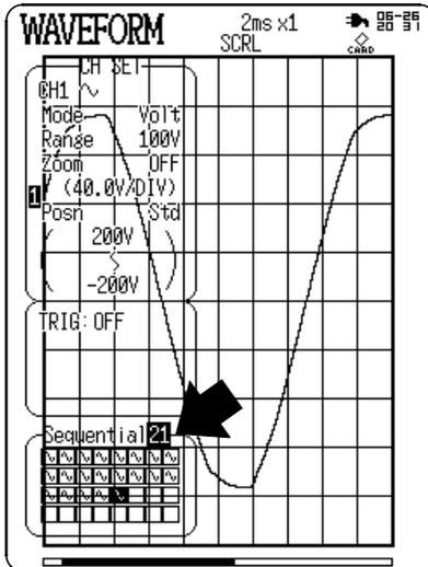
When measurement is restarted, all previous waveforms are deleted and recording commences from the first block.
