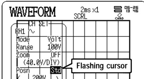
Pressing the POSN key moves the flashing cursor automatically to the Time Axis position for setting.
