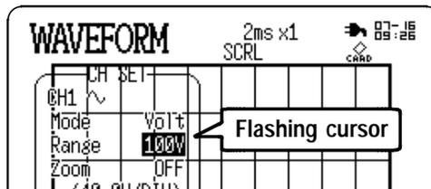
Pressing the RANGE key moves the flashing cursor automatically to the Time Axis position for setting.
