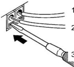
1. Push the tab with a flatblade screwdriver or similar.
