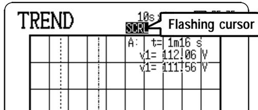
3. Move the cursor using the ◀ ▶ scrolling key to scroll the display. Pressing the ◀ / ▶ keys scrolls faster.
