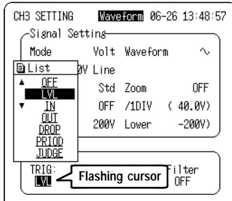
3. Move the flashing cursor to the position shown in the figure below, and set the trigger level using the ▲/▼ keys.
