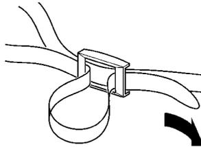
3. Finally, slide the stopper over the end of the strap. Tighten the strap to remove slackness or twisting.
