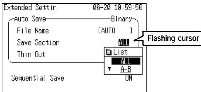
Move the flashing cursor to the position shown in the figure below and use the ▲/▼ keys to make a setting.
