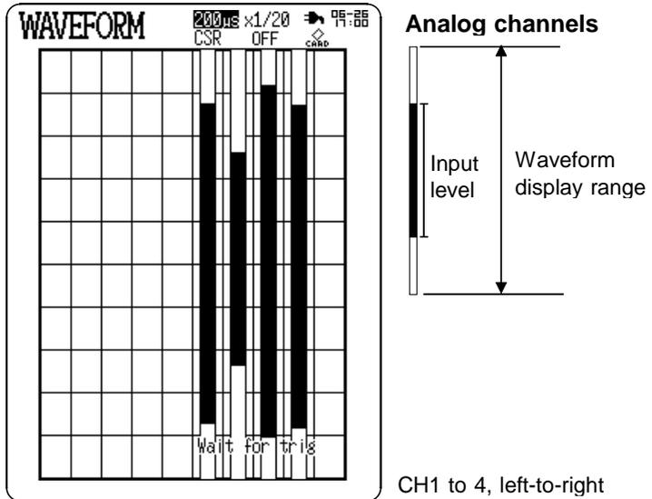
When the input level is not displayed on the screen display range
