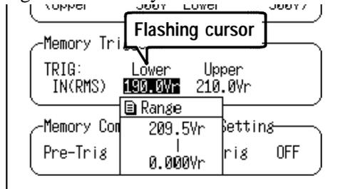
4. Move the flashing cursor to the upper limit, and set the upper limit of the trigger level using the ▲/▼ keys. The upper limits must not be smaller than the lower limits, or the lower limits must not be larger than the upper limits.
