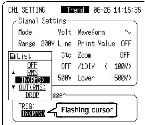
3. Move the flashing cursor to the position shown in the figure below, and set the lower limit of the trigger level using the ▲/▼ keys.
