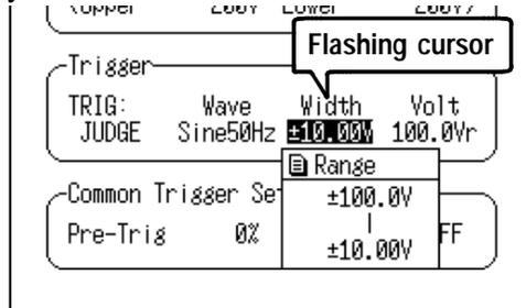
5. When 50- or 60-Hz Sine Wave was selected in step 3, set the Standard Voltage.
