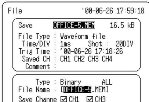
5. Move the flashing cursor to the File name, and press the DMM key twice. The file name selected in step 3 entries in the File Name entry location.
