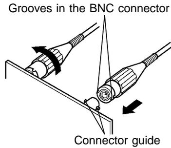
1. Align the grooves in the BNC connector with the guide pins on the instrument input connector, then turn clockwise while pressing in to lock the connector.
