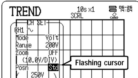
Pressing the POSN key moves the flashing cursor automatically to the Time Axis position for setting.
