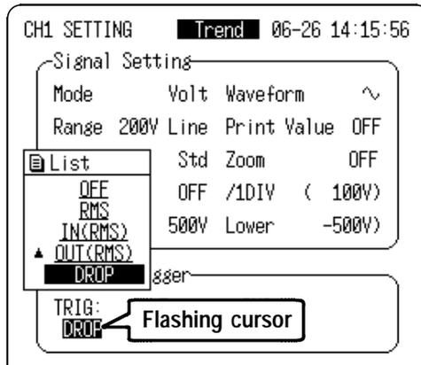
3. Move the flashing cursor to the position shown in the figure below, and set the frequency to be measured using the ▲/▼ keys.
