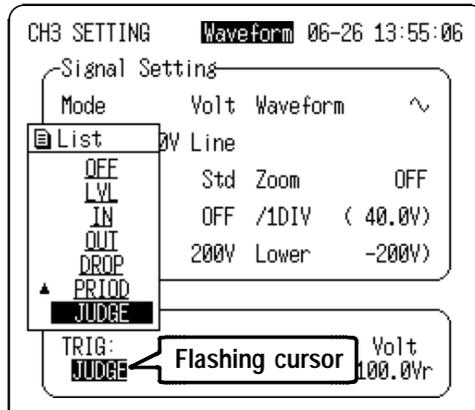
3. Move the flashing cursor to the position shown in the figure below and select the reference waveform using the ▲/▼ keys.
