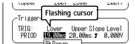
4. Move the flashing cursor to the upper limit, and set the upper limit of the trigger level (period range) using the ▲/▼ keys.
