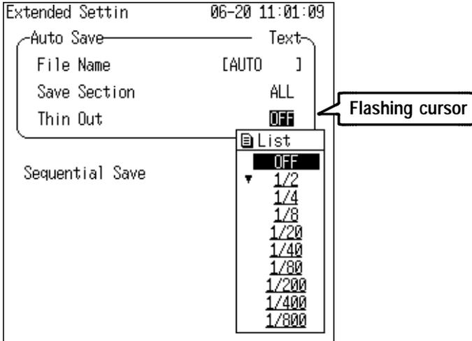
Move the flashing cursor to the position shown in the figure below and use the ▲/▼ keys to make a setting.
