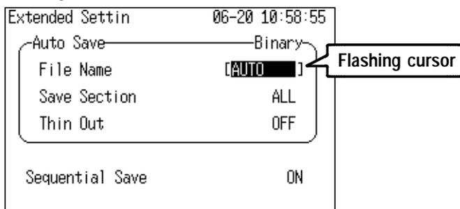
If the file name entered as a blank [        ], it is assigned automatically according to the following principle.
