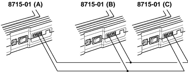
When the trigger conditions of the 8715-01 (A) are met and the trigger is activated, a pulse signal is output from the trigger output terminal.
