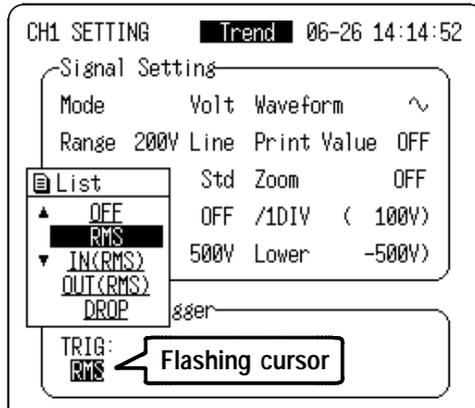
3. Move the flashing cursor to the position shown in the figure below, and set the trigger level using the  $\blacktriangle$ / $\blacktriangledown$  keys.
