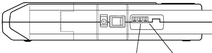
Trigger output terminal    GND terminal
