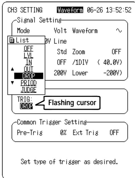
3. Move the flashing cursor to the position shown in the figure below, and set the frequency to be measured using the ▲/▼ keys.
