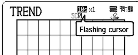
Pressing the TIME/DIV key sets the time axis regardless of the flashing cursor position.
