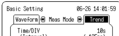
With the RMS Trend Mode (rms recording), the rms value is continuously recorded in real time from the moment the START key is pressed to start measuring until the STOP key is pressed.
