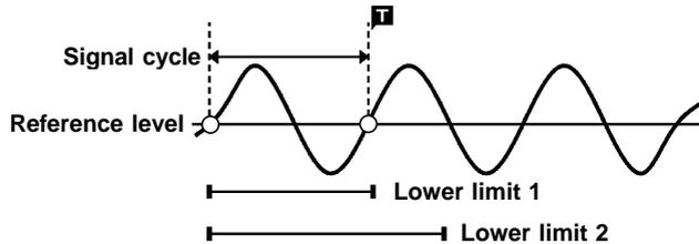
When the signal crosses the reference level at the set trigger slope before the lower limit of the set period range appears on the screen, the intersection is always defined as the triggering position.
