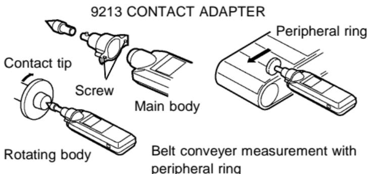
1. Attach the contact adapter over the detector window with the "up" mark facing up. Tighten it with a screwdriver on both sides.
