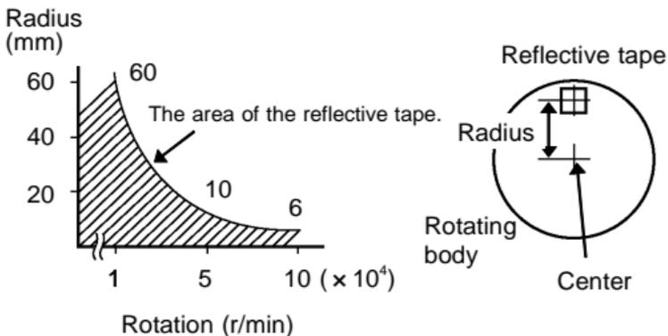
If the reflective tape cannot be attached within this detection range, increase the area of the reflective tape so that the generated pulse is 0.2 ms or higher.
