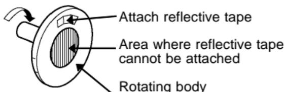
For measurement of 30,000 r/min or higher, use the following method:
