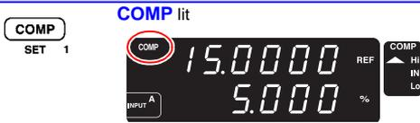
The comparator measurement function is enabled. Pressing the COMP key executes comparator decision according to the settings
