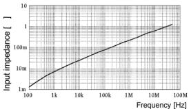
Figure 3 Input impedance (Characteristics)
