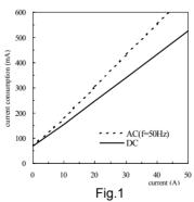
Current consumption\* vs. current to be measured(typical)
