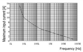
Figure 2 Derating according to frequency
