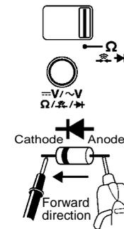
1. Move the Function Selector to the  $\rightarrow$  position and press the select button twice. ( $\rightarrow$  lights up) (During manual ranging, press the select button for at least 1 second.)
