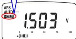
To cancel the trigger hold function, press and hold the **REC/HOLD** key.
