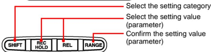
1. In order to display the setting screen hold down the **SHIFT** key and turn the unit on by turning the function switch from the OFF position.
