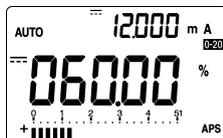
$$\text{Percentage conversion value} = \frac{\text{Measured value[mA]}}{20[\text{mA}]} \times 100[\%]$$
