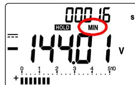
3. To clear the maximum value, minimum value and update time and restart, press the **DUAL** key. To cancel the peak hold function, hold down the **REL** key.
