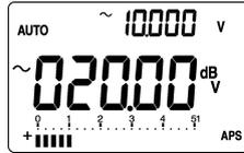
$$\text{dBV} = 20 \log_{10} (\text{Measured value [V]}) \quad [\text{dBV}]$$
