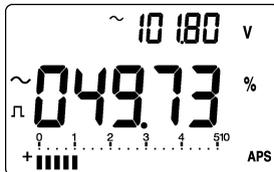
To switch the pulse slope polarity  $\sqcup$   $\sqcap$ , hold down the **SHIFT** key.
