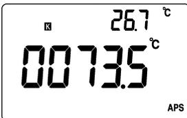
1. Select the thermocouple sensor (K or J).
