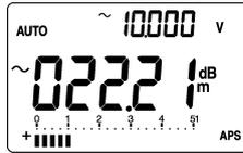
$$\text{dBm} = 10 \log_{10} \frac{(\text{Measured value [V]})^2 \times 1000}{\text{Reference resistance } [\Omega]} \quad [\text{dBm}]$$
