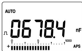
The sample rate for the 99.99 mF range is 0.01 times/second. It may take as long as two minutes before the measured value is displayed. This instrument measures capacitance by the charge-discharge method.  $\sqcup \sqcup$  on the display indicates that the capacitor is charging ( $\sqcup$ ) / discharging ( $\sqcup$ ).
