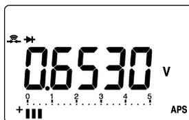
With a normal diode, the sequential order voltage (0.3 to 0.8 V) is displayed. When the display value less than 0.0500 V, buzzer sounds.
