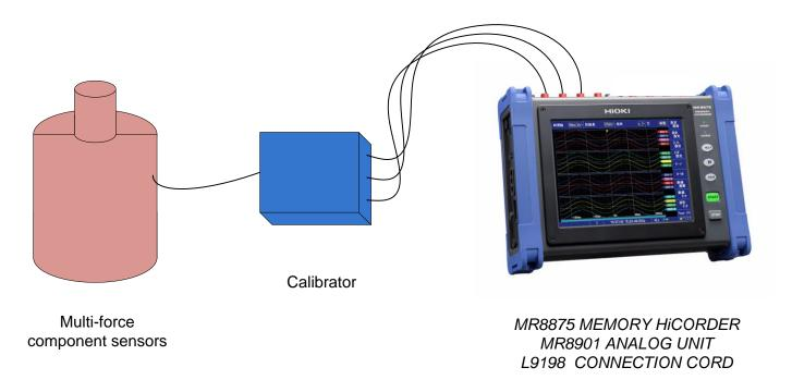
This is an example of recording the output of a three-force component sensor with the MR8875 Memory HiCorder.
