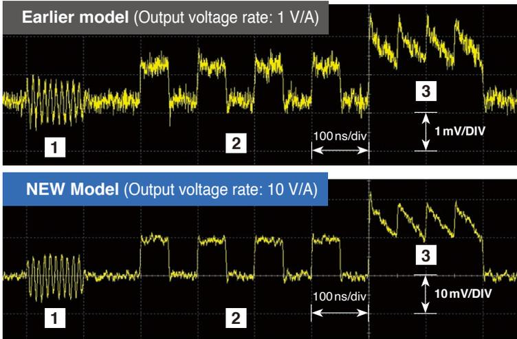
By improving voltage sensitivity of the oscilloscope by a factor of 10, the S/N ratio of the oscilloscope itself is enhanced to deliver a cleaner waveform.
