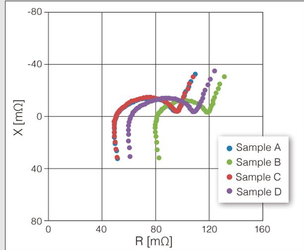
The above diagram contains Cole-Cole plots for new battery cells of the same kind. A and C have almost consistent impedance characteristics. Due to having impedance greater than A and C, B and D produce heat and deteriorate first when they are used within the same battery pack.
