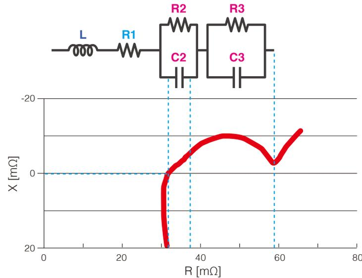
The impedance characteristics of a Cole-Cole plot are generally expressed as a pseudo equivalent circuit.
