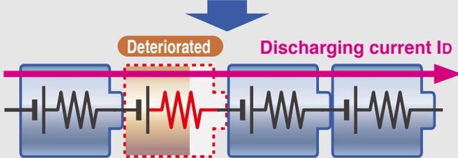
The protective circuit works based on the cell with the lowest capacity, reducing the discharging capacity of the entire battery pack as a result.
