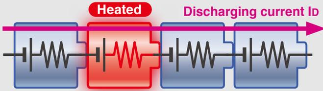
If the resistance of the battery pack is different, some of the batteries will heat up excessively, thereby lowering the capacity and accelerating deterioration.
