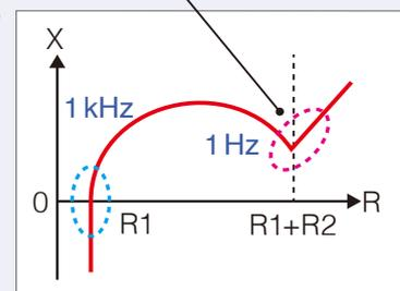
Electrolyte resistance and welding resistance
