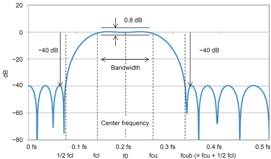
Where the center frequency of the band-pass filter is  $f_0$  and the bandwidth is  $f_w$ , the lower pass-band edge ( $f_{cl}$ ) and the upper pass-band edge ( $f_{cu}$ ) are calculated by the following expressions:
