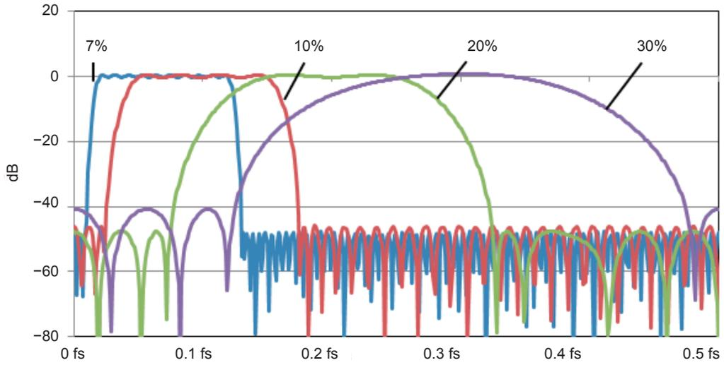
Example of FIR-BPF frequency characteristics (bandwidth: 15%)
