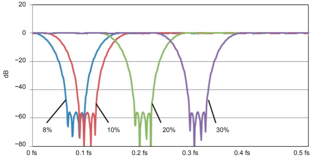
Example of FIR-BSF frequency characteristics (bandwidth: 20%)
