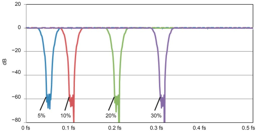
Example of FIR-BSF frequency characteristics (bandwidth: 10%)
