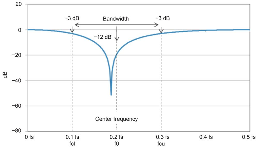
The bandwidth that can be set for the IIR band-stop filter varies depending on the center frequency.
