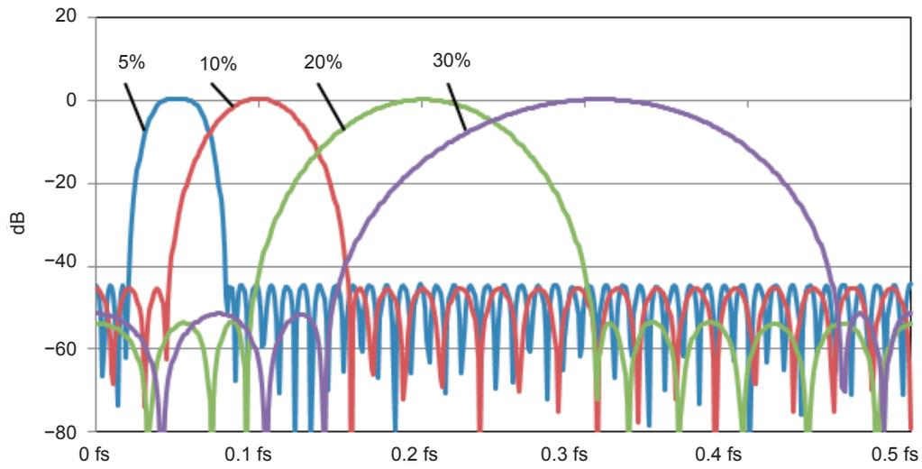
Example of FIR-BPF frequency characteristics (bandwidth: 5%)
