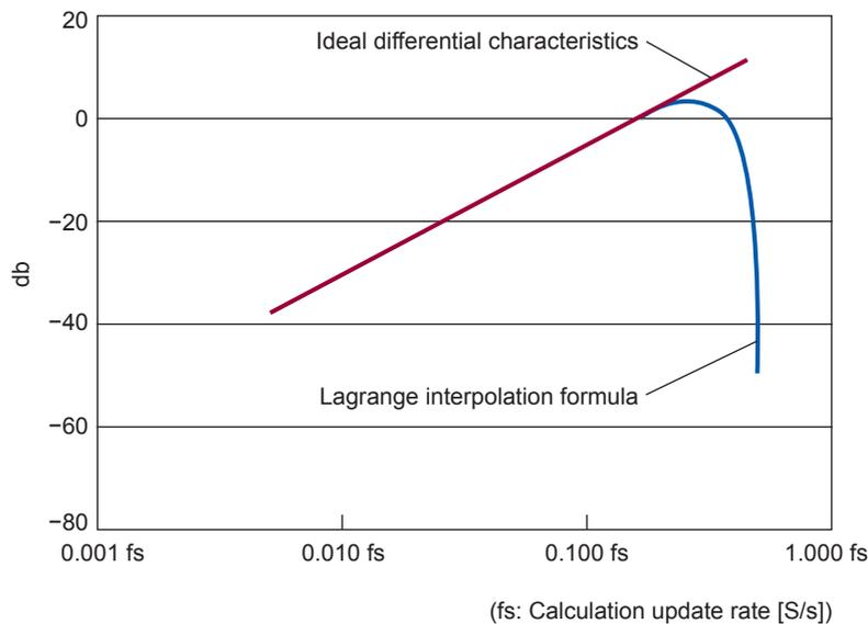
When an input frequency is within 20% of the calculation period, the differential characteristics is nearly equal to ideal differential characteristics. Frequency components higher than the above are suppressed due to the high range characteristics of Lagrange interpolation formula.
