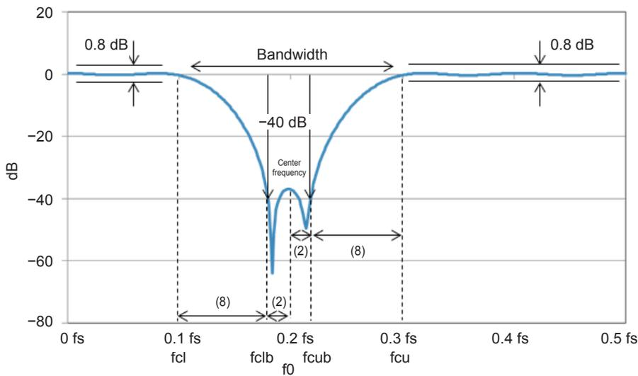
The bandwidth that can be set for the FIR band stop filter varies depending on the center frequency.
