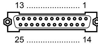
9670 Printer (25-pin) Connector (Example)
