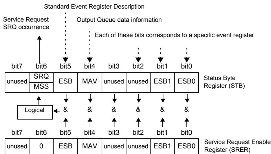
The Status Byte Register contains information about the event registers and the output queue. Required items are selected from this information by masking with the Service Request Enable Register. When any bit selected by the mask is set, bit 6 (MSS; the Master Summary Status) of the Status Byte Register is also set, which generates an SRQ (Service Request) message and dispatches a service request.
