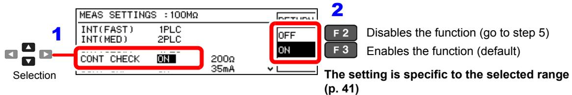
**4** Select the contact check fault threshold resistance.
