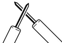
**4 Confirm that the measured value does not exceed 10 Ω.**
