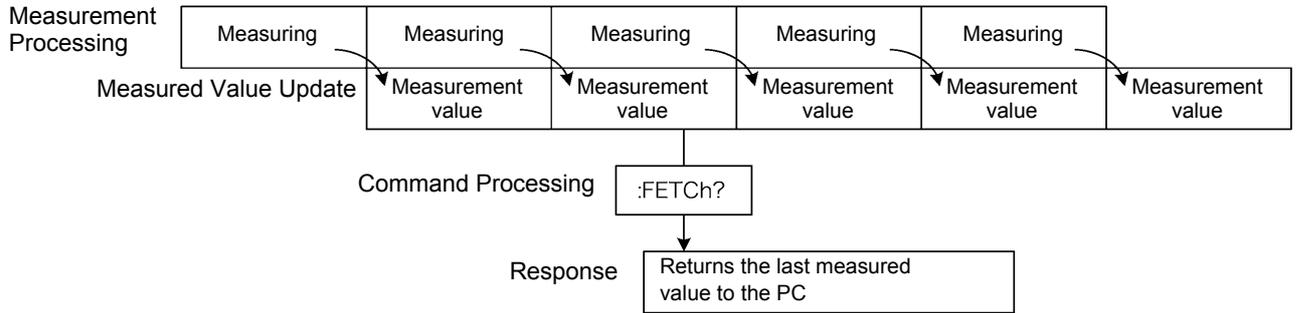
This is the simplest method for exporting measured values. It is ideal when measurement (tact) time is not limited, and when external synchronization is not needed. After connecting to the measurement object, wait for twice the measurement time plus the self-calibration time (about 130 ms) before exporting the measured value.
