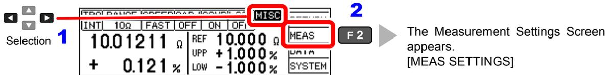
**3** Enable the Contact Check function.
