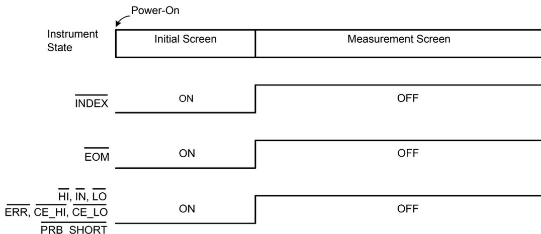
Operation is shown when the trigger source is set to external triggering (EXT).
