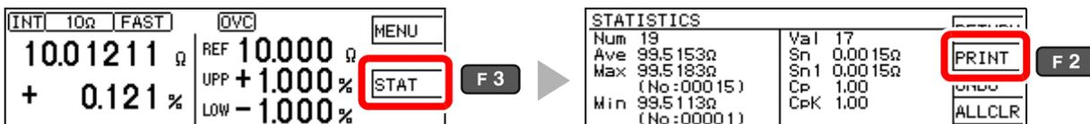
If no valid data exists, only the data count is printed. When only one valid data sample exists, standard deviation of sample and process capability indices cannot be printed.
