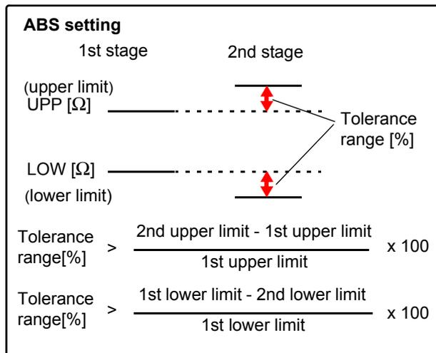
4.9 Comparing the Measurement Settings of Two Instruments (Settings Monitor Function)
