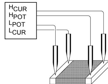
Figure. 11 Four-Terminal Measurement
