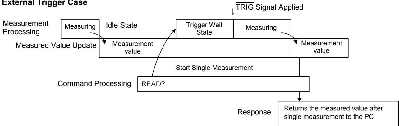
Use this method to measure (and export) synchronously with the PC or external trigger signal. Measurement time can be minimized.
