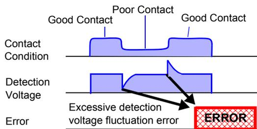
**Reliable Four-Terminal Measurement – Probe Short-Circuit Detection Function (p. 51)**
