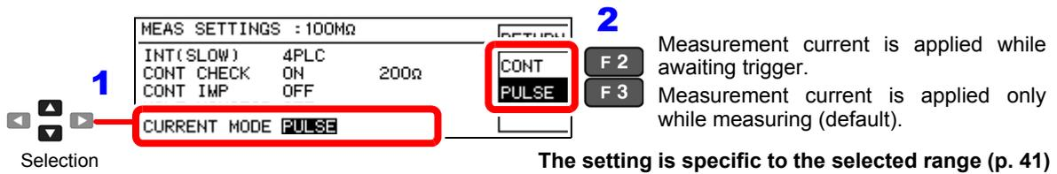
To apply measurement current continuously (CONT setting) even when waiting for a trigger, confirm that the Contact Improver function is disabled (CONT IMP: OFF, (p. 47)).
