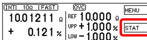
When statistical calculation is enabled, **F3** [STAT] appears on the Measurement screen.
