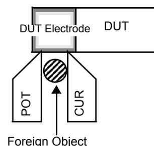
When a probe short-circuit is detected, an error message appears on the measurement screen, and the  $\overline{\text{PRB\_SHORT}}$  and  $\overline{\text{ERR}}$  signals are output. (**ERR:021 Probe short error**)
