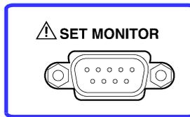
The SET MONITOR connectors are identical to RS-232C connectors. Be careful to avoid connecting the wrong connectors.
