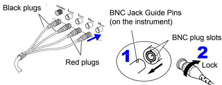
Connect the red plugs to the  $H_{CUR}$  and  $H_{POT}$  jacks, and the black plugs to the  $L_{CUR}$  and  $L_{POT}$  jacks.
