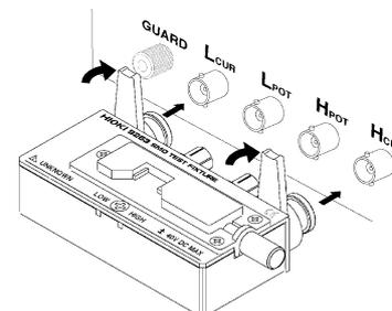
Connect directly to the measurement jacks with the label side up, and affix with the levers on the left and right.
