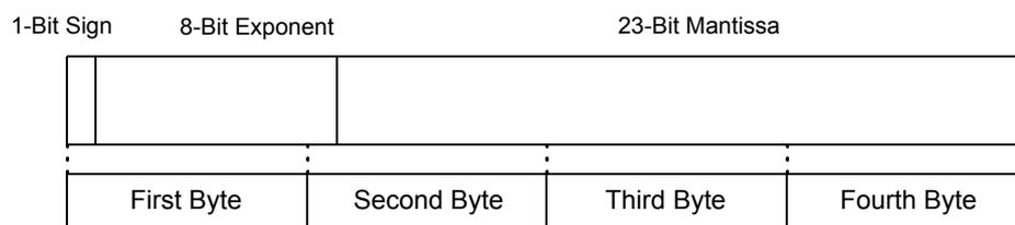
Binary data is sent in four-byte sequences beginning with the first byte (which includes the sign bit).
