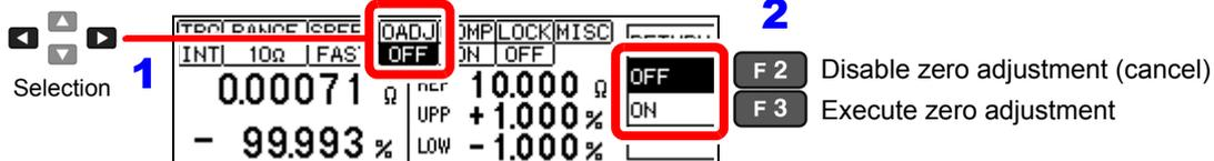
After confirming that the measured value does not exceed 10 Ω, execute zero adjustment.
