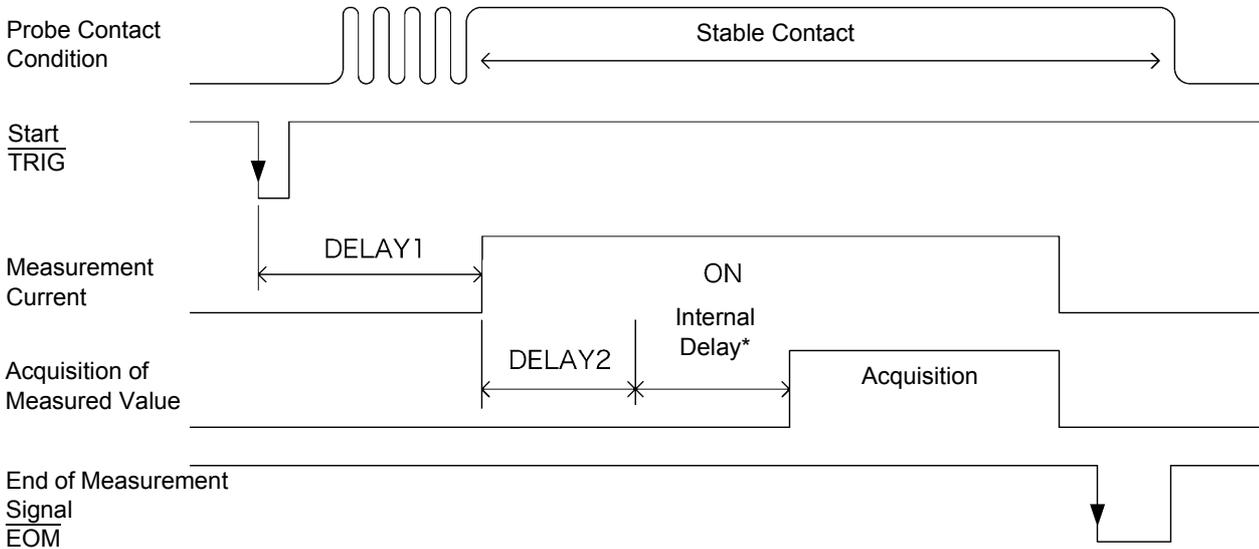
\* Internal delay is provided to suit purely resistive (non-reactive) DUTs, and is different for each measurement range.
