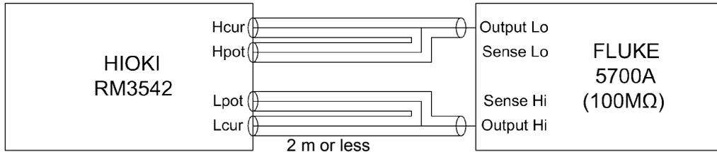
Calibration using Fluke 5700A at 100 MΩ
