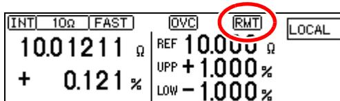
In the local lockout state (GP-IB command LLO: Local Lock Out, (p. 114)) selecting [LOCAL] on the screen has no effect. In this state, send the GTL command, or turn the instrument off and back on to re-establish local control. If the Setting screen was displayed when remote control was enabled, the instrument returns to the Measurement screen automatically.
