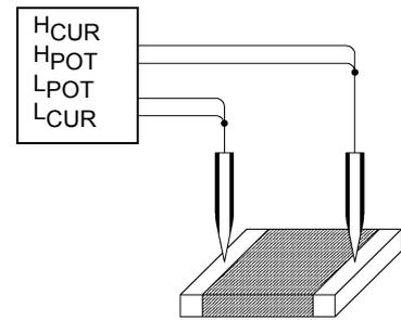
Figure. 10 Two-Terminal Measurement
