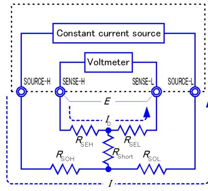
$$\begin{aligned} E &= (I_0 \times R_{SEL}) + (I_0 \times R_{SEH}) \\ &= (0 \times R_{SEL}) + (0 \times R_{SEH}) \\ &= 0 [\text{V}] \end{aligned}$$
