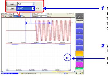
Move the cursor to the [Load] setting item, and select the location (division number) of the measurement waveform to display.
