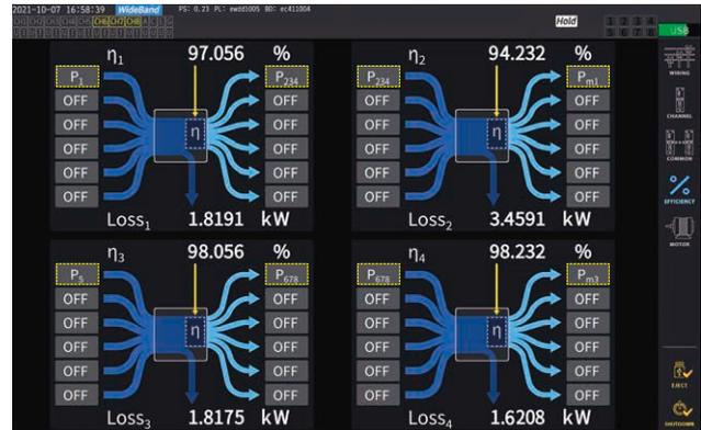
The results indicate that the front motor (Pm1) has a somewhat low efficiency of 94.2% and that 3.4 kW of loss is occurring.
