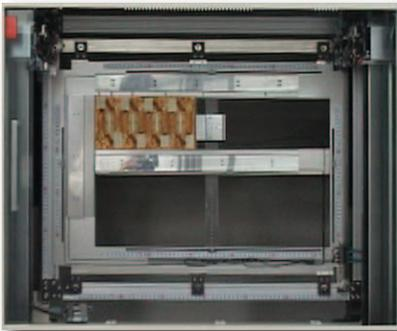
Fixing flexible boards with tension frames
