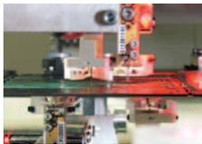
**• Elimination of contact errors through automatic board thickness correction and tension features**
