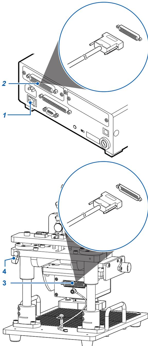
**1** Verify that the RM2611 Electrode Resistance Meter's main power switch (on the rear of the instrument) is in the OFF (○) position.
