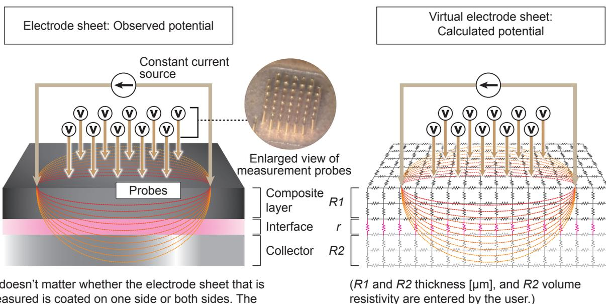
(It doesn't matter whether the electrode sheet that is measured is coated on one side or both sides. The composite layer resistivity and interface resistance on the probed surface are output.)
