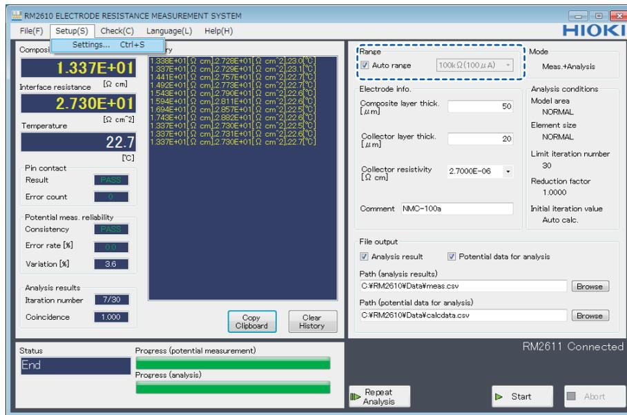
To indicate that potential measurement results obtained using the 10 MΩ range are merely values for reference purposes, values of the composite layer volume resistivity and interface resistance appear dimmed.
