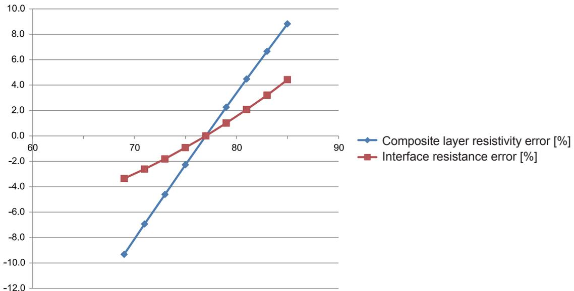
Figure: Effects of incorrectly entering the thickness (representative example for a positive electrode)
