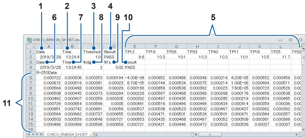
**RM9004 Test Fixture OPEN inspection results file format**
