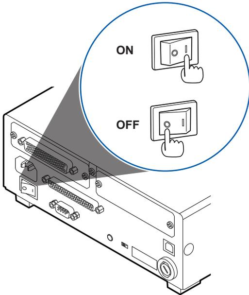
Place the RM2611 Electrode Resistance Meter's main power switch (on the rear of the instrument) in the ON (|) or OFF (○) position.
