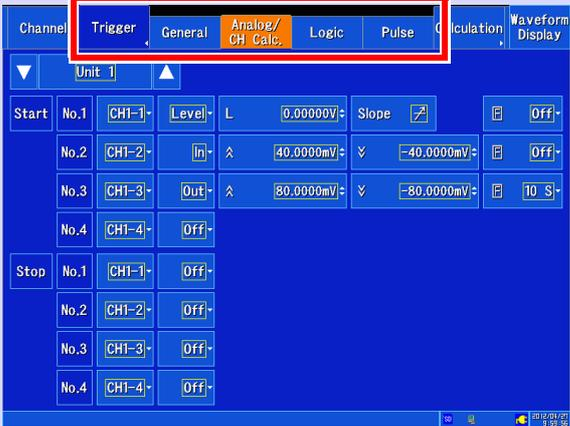
The Trigger screen has a menu bar with Channel, Trigger, General, Analog/CH Calc., Logic, Pulse, Calculation, and Waveform Display. The 'Analog/CH Calc.' option is circled in red. The main area shows a table for configuring trigger levels and slopes for four channels.
