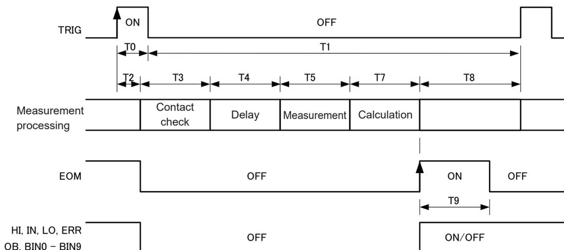
**(3) When the trigger source is set to INTERNAL while the instrument is in the RUN state**
