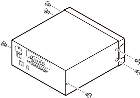
**1** Verify that the power to the instrument is OFF and unplug the power cord, and any other cords or cables.
