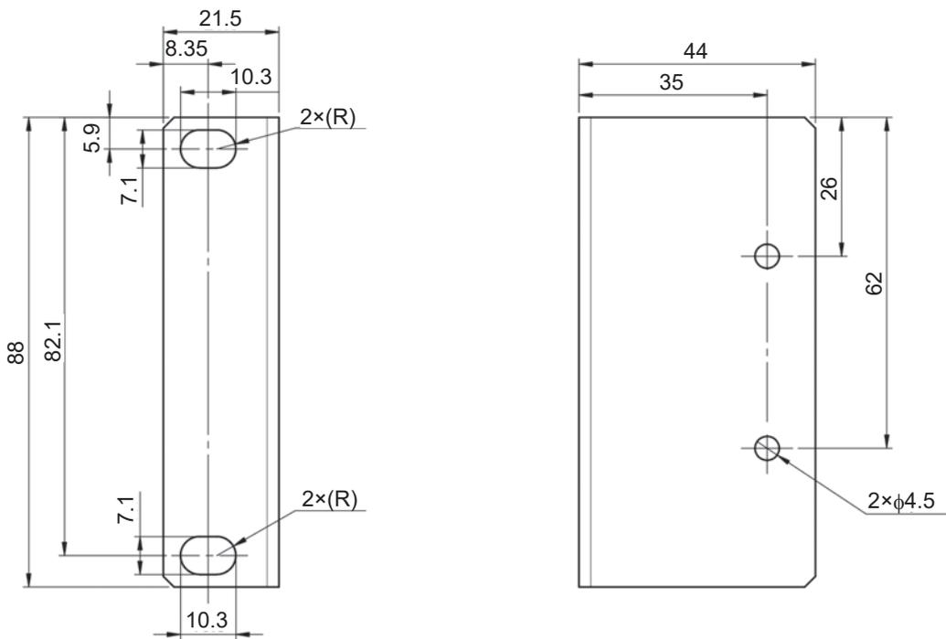
**Rack-mounting bracket (JIS-compliant, to mount 1 instrument)**
