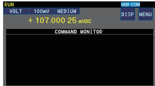
The communications monitor is displayed on the Measurement screen.
