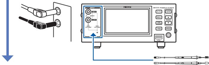
(5) Connect the temperature sensor to the TEMP.SENSOR connector. (When performing temperature measurement or using the temperature compensation function) (p.27)
