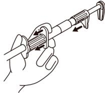
**2** Open the clip by depressing as you would the plunger of a syringe.
