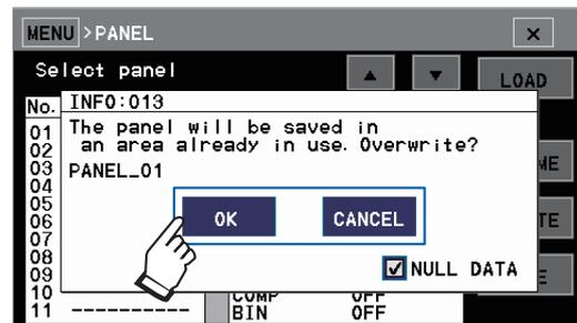
Touch **OK** to overwrite the previously saved data with the current measurement conditions.
