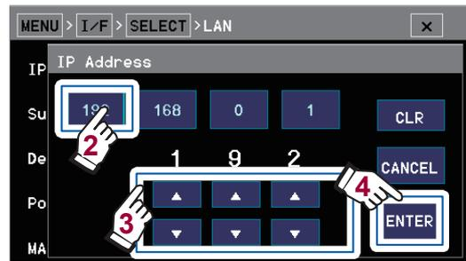
Set the IP address, subnet mask, gateway, and communications command port.
