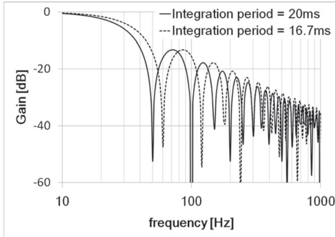
Figure 6. Noise Rejection Characteristics Using Integration
