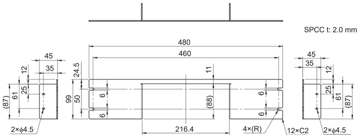
**Rack-mounting bracket (JIS-compliant, to mount 2 instruments)**
