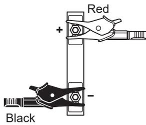
Connect, taking care to align the measurement cable colors with the measurement target's polarity. Clip at the middle of the clip.
