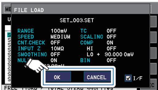
Touch **OK** to replace the instrument's settings with the loaded measurement settings.
