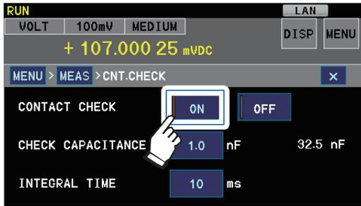
Enable the contact check function.
