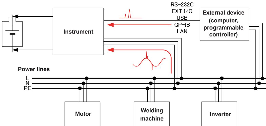
Figure 1. Ingress of Conductive Noise
