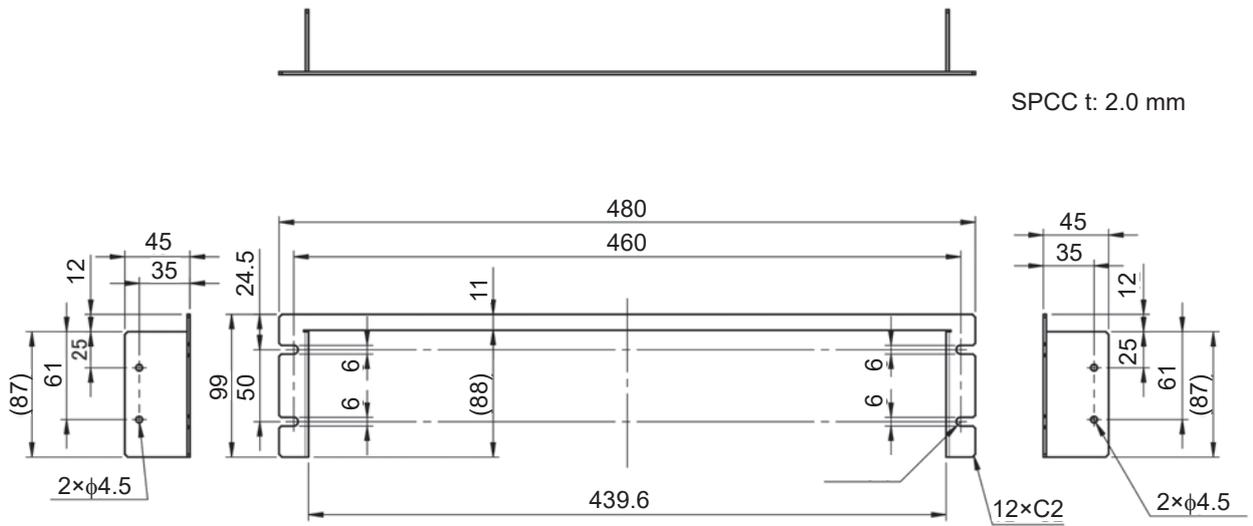
**Connecting bracket (EIA- and JIS-compliant)**
