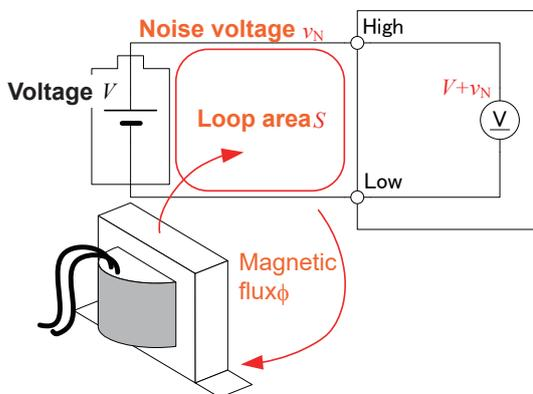
Figure 3. Noise Coupling from a High-current Circuit
