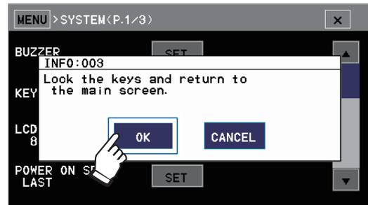
The key lock function will be enabled, and the display will return to the Measurement screen.
