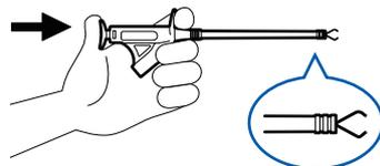
**2** Open the tip of the clip by depressing as you would the plunger of a syringe.
