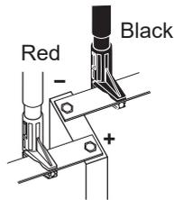
**3** Connect, taking care to align the measurement cable colors with the measurement target's polarity.
