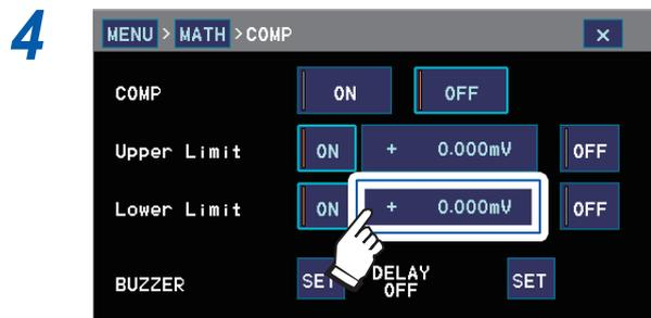
**4 Enter a lower limit value using the same method as for the upper limit value.**
