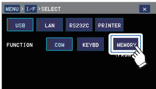
When **USB COM** or **USB KEYBD** is selected, data cannot be saved on a USB flash drive.
