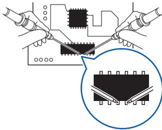
L4933 pin diameter:  $\phi 1.0$  mm
