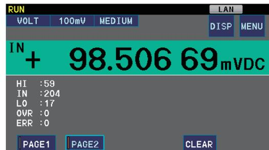
The count for each judgment result, the number of measured values outside the measurement range, and the number of errors are shown.
