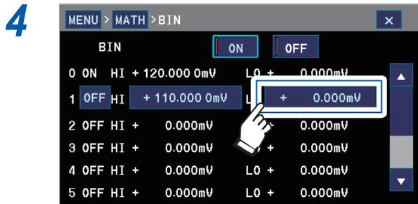
**Enter a lower limit value using the same method as for the upper limit value.**
