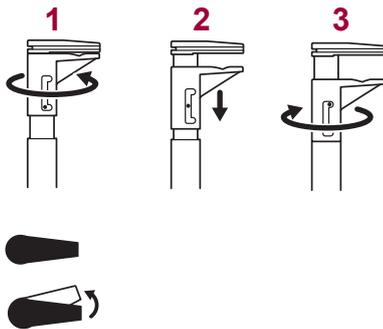
To apply the clip to a thick target:
