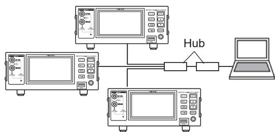
In addition, you can control the instrument using communications commands by creating a program and having it connect to the communications command port using TCP. (See the Communication Command Instruction Manual on the included application disc.)
