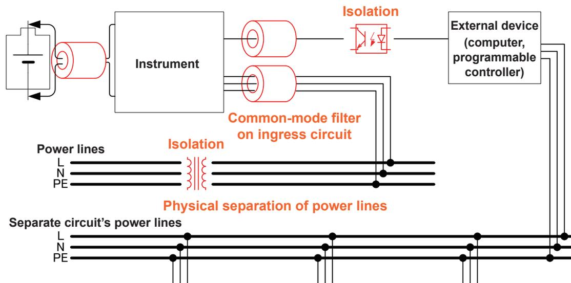
Figure 2. Conductive Noise Countermeasures
