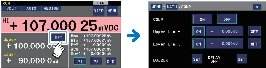
The screen display varies with the combination of comparator measurement and BIN measurement.
