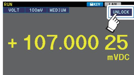
While the key lock function is enabled, the **KEY** icon will be displayed at the top of the screen.
