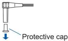
Each test lead plugs is covered by a protective cap.
