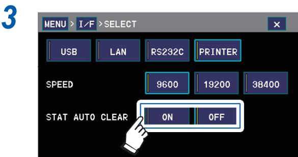
**ON** Automatically clears the statistical calculation results every time they are printed.
