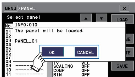
Touch **OK** to replace the current settings with the settings in the loaded panel data.
