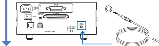
(6) Configure and connect the external interface (as necessary).
