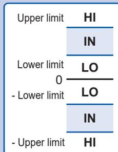
When (lower limit value  $\leq$  |measured value|  $\leq$  upper limit value), the instrument will generate an IN judgment.
