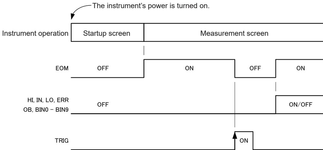
The above chart depicts instrument operation when the trigger source is set to **EXTERNAL** and EOM output is set to **HOLD**.
