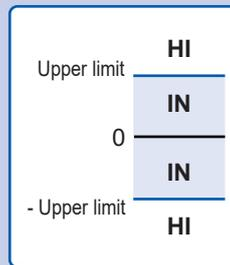
When (|measured value|  $\leq$  upper limit value), the instrument will generate an IN judgment.
