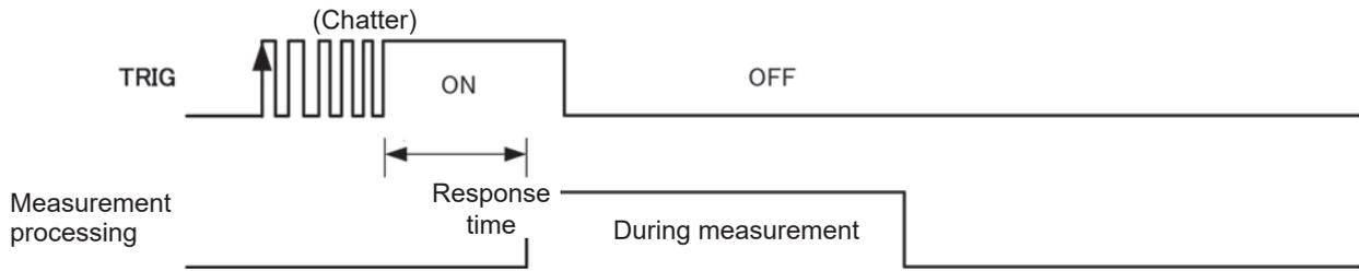
Hold the input signal until the response time has passed.
