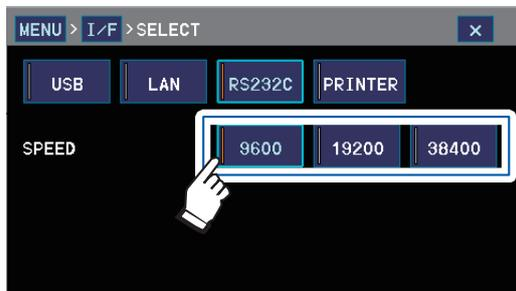
Select the transfer speed (baud rate).
