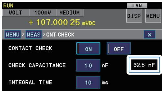
If the capacitance monitor value is the same as the contact check threshold, the instrument may either detect a contact error or display the measured value.
