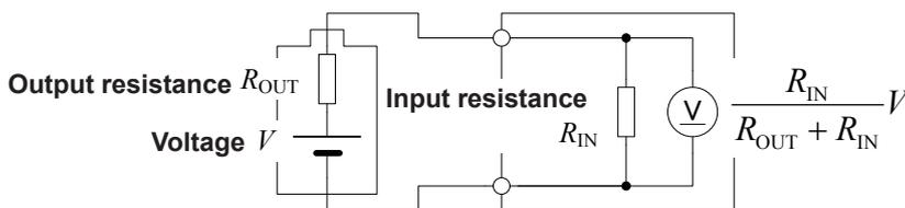
Figure. Effects of Input Resistance
