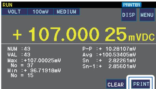
If there is no valid data, only the number of data points will be printed. If there is one valid data point, the sample standard deviation and process capability index will not be printed.
