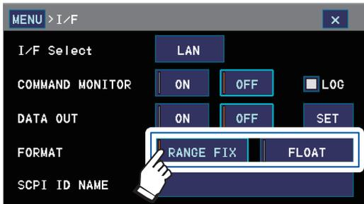
**RANGE FIX** Fixes the exponent part based on the measurement range (default setting).
