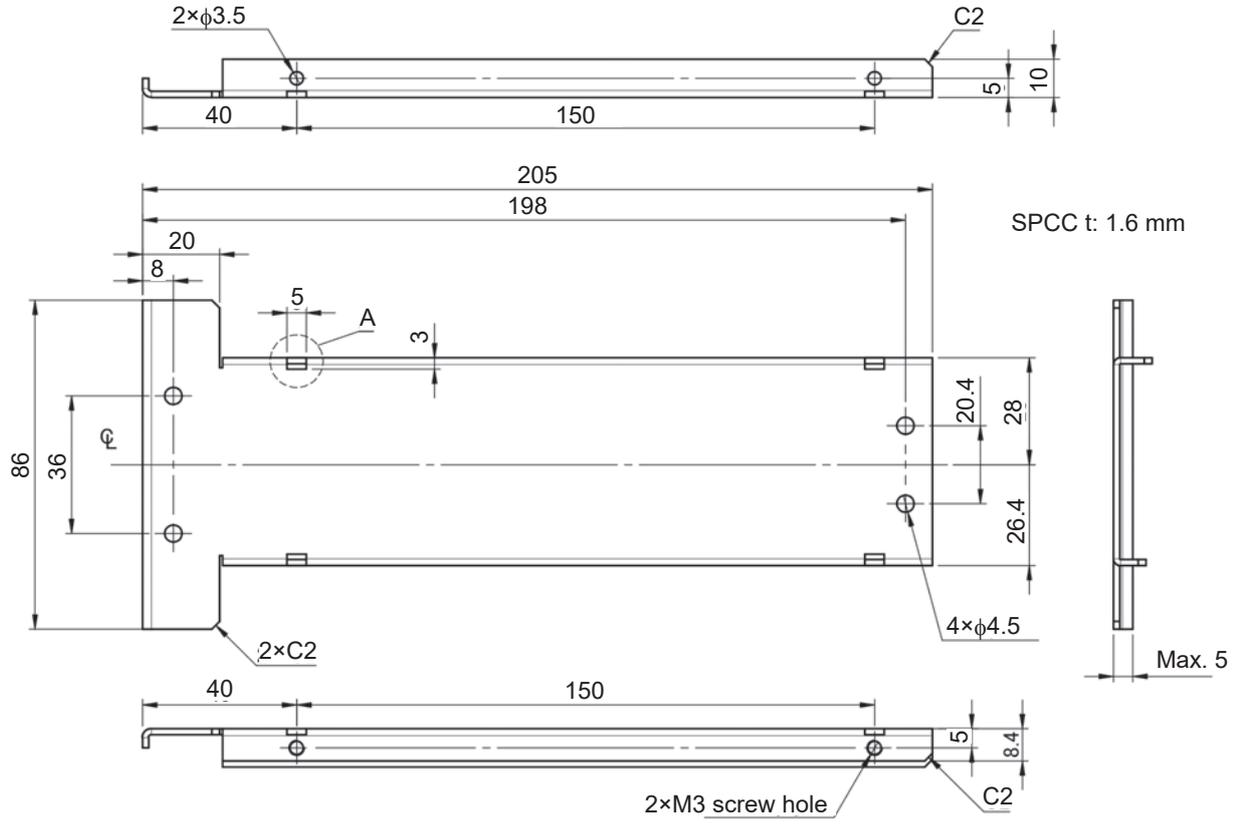
Notches (one of which can be found in area labeled A) serve to prevent distortion of the shape of the hole caused by flexing (total of four).
