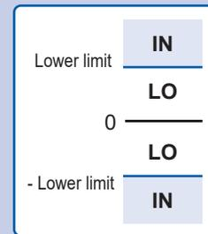
When (|measured value|  $\geq$  lower limit value), the instrument will generate an IN judgment, including in the event of an over-range (**+OvrRng/-OvrRng**) event.
