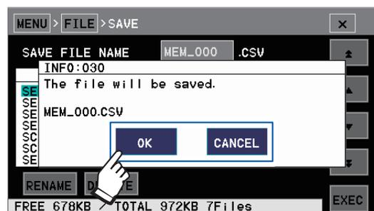
Touch **OK** to output the measurement data to the USB flash drive.
