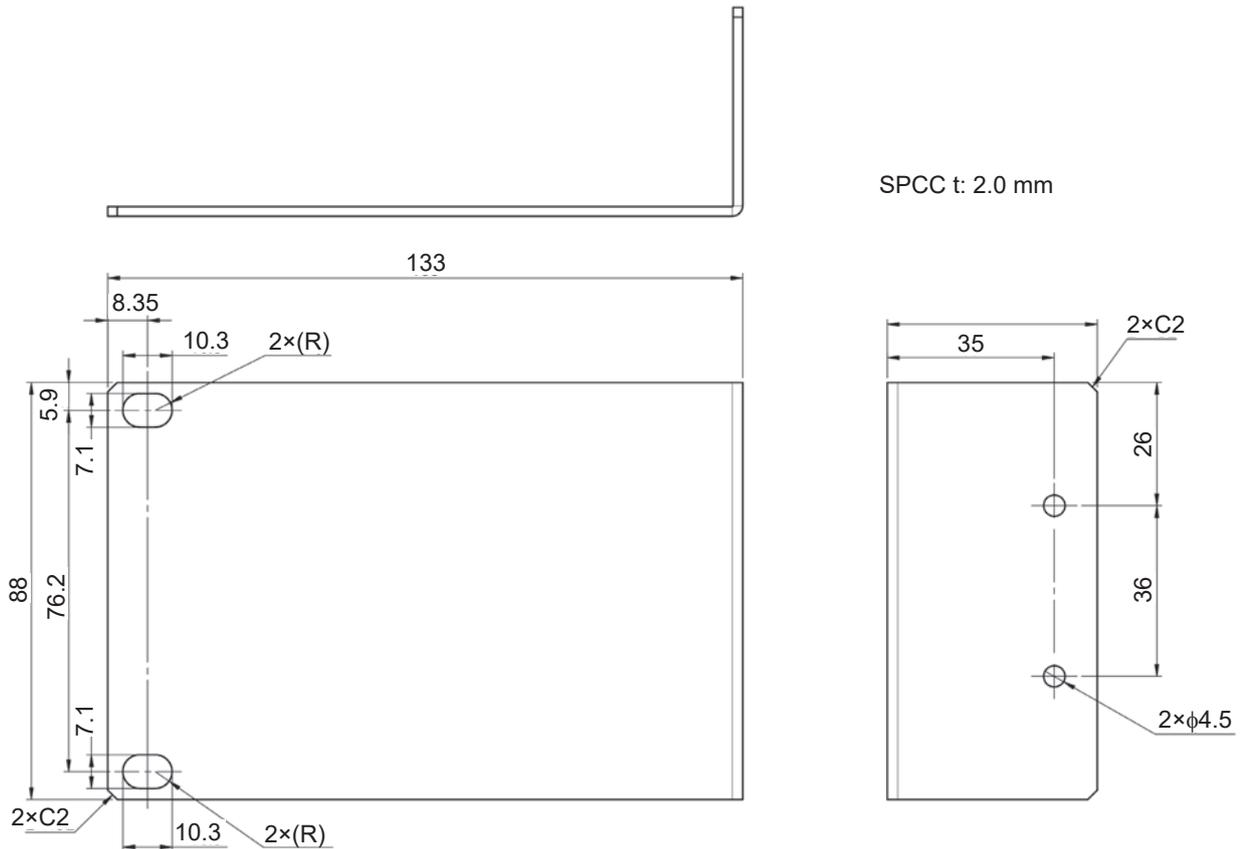
**Rack-mounting bracket (EIA-compliant, to mount 2 instruments)**
