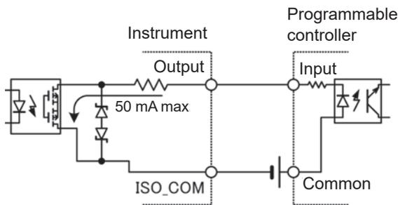
Connection to programmable controller (positive common input)
