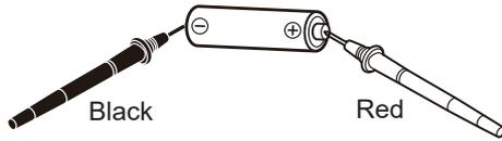
Connect, taking care to align the measurement cable colors with the measurement target's polarity.
